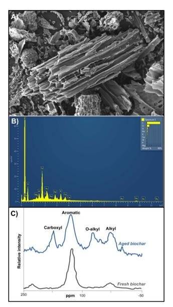
Fig. 4 Hardwood-derived biochar (BC) characterised by scanning electron microscopy – SEM (A) and energy dispersive X-ray spectroscopy – EDX (B), with a solid-state <sup>13</sup>C CP-MAS NMR spectra of fresh and aged BC (C). Reproduced (adapted) with permission from ref. 78 Copyright© 2015, Taylor & Francis, and Ondrasek *et al.*, unpublished Kliknite ili dodirnite ovdje da biste unijeli tekst.
