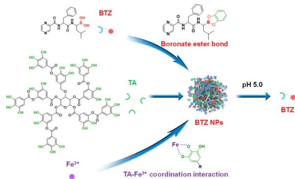
**Scheme 1** Schematic illustration for the preparation of BTZ NPs by the self-assembly of BTZ, TA, and Fe<sup>3+</sup>. The release of BTZ could be realized in an acidic environment.
