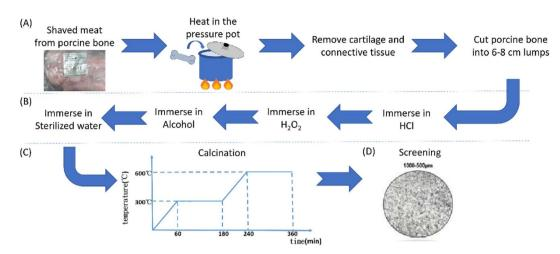
Fig. 1 Protocol for a porcine bone graft. (A) Pre-treatment, (B) acid treatment, (C) calcination, and (D) the finished porcine graft.
