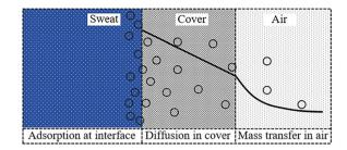
Fig. 2 Schematic diagram of the dissolution diffusion model.
