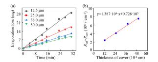
Fig. 7 (a) Evaporation loss of water through PET membrane under different cover thicknesses of microfluidic patches. (b) The relationship between the sum of interface resistance and diffusion resistance and the thickness of the PET cover of microfluidic chips.
