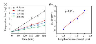
Fig. 8 (a) Water evaporation loss along microchannel under different channel lengths. (b) The relationship between the diffusion resistance of the microchannel and the channel length.
