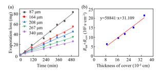
Fig. 6 (a) Evaporation loss of water through PDMS membrane under different cover thicknesses of microfluidic patches. (b) The relationship between the sum of interface resistance and diffusion resistance and the thickness of the PDMS cover.
