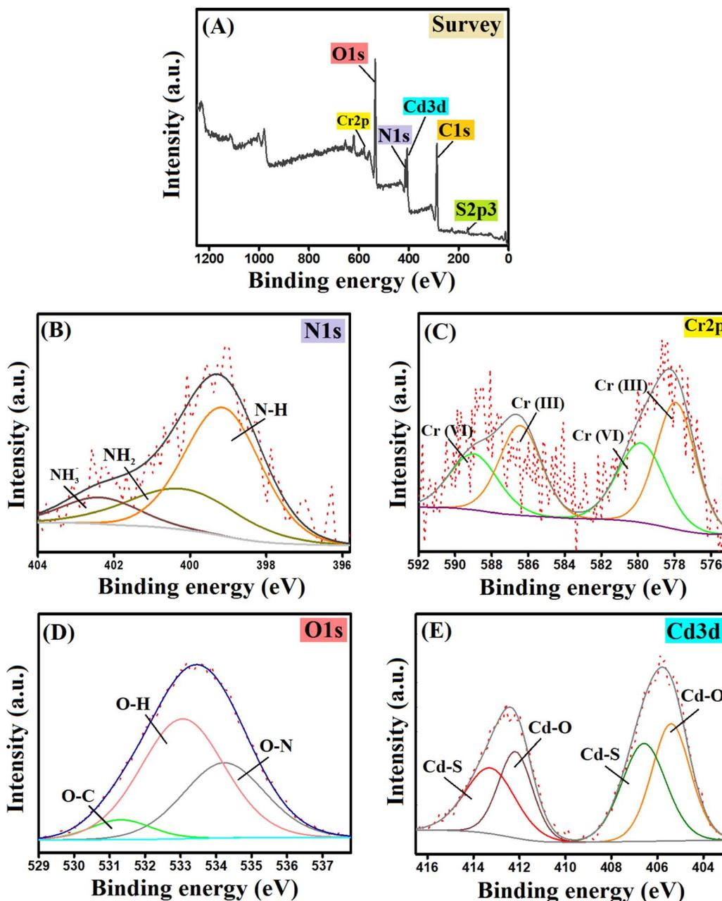
Fig. 7 The XPS spectra of the Cr(vi)-adsorbed CdS/PEI-BC/CTS composite: (A) survey, (B) N 1s, (C) Cr 2p, (D) O 1s, and (E) Cd 3d.
