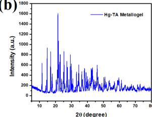
Fig. 6  $\,$  (a and b) PXRD spectra of Cd–TA and Hg–TA metallogel in their xerogel form.
