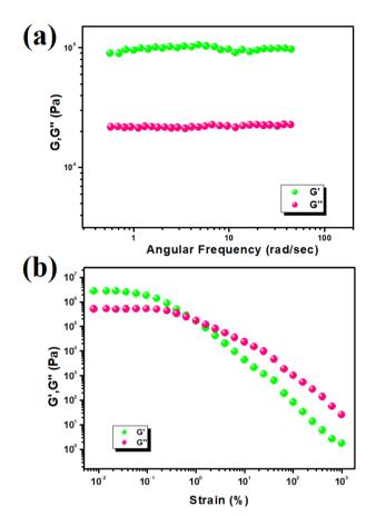
Fig. 3 (a) The figure depicts the relationship between the storage modulus (G') and loss modulus (G'') of Hg(II) metallogel as a function of angular frequency; (b) strain-sweep measurements of Hg(II) metallogel were carried out at a steady frequency of 6.27997 rad s<sup>-1</sup>
