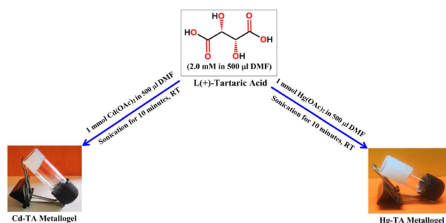
Fig. 1 Schematic representation of the synthetic route of Cd(II)-metallogel (Cd-TA) and Hg(II)-metallogel (Hg-TA).
