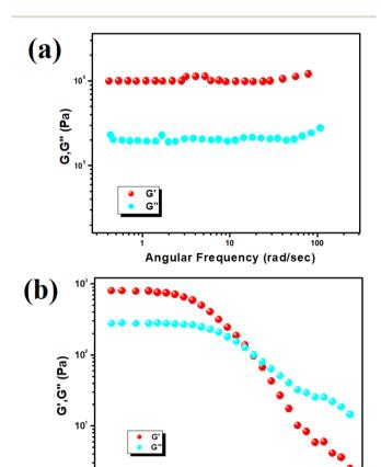
Fig. 2 (a) The graph illustrates the variation of storage modulus (G') and loss modulus (G'') of Cd( $\shortparallel$ ) metallogel with angular frequency; (b) strain-sweep measurements of Cd( $\shortparallel$ ) metallogel were conducted at a consistent frequency of 6.283 rad s<sup>-1</sup>.
