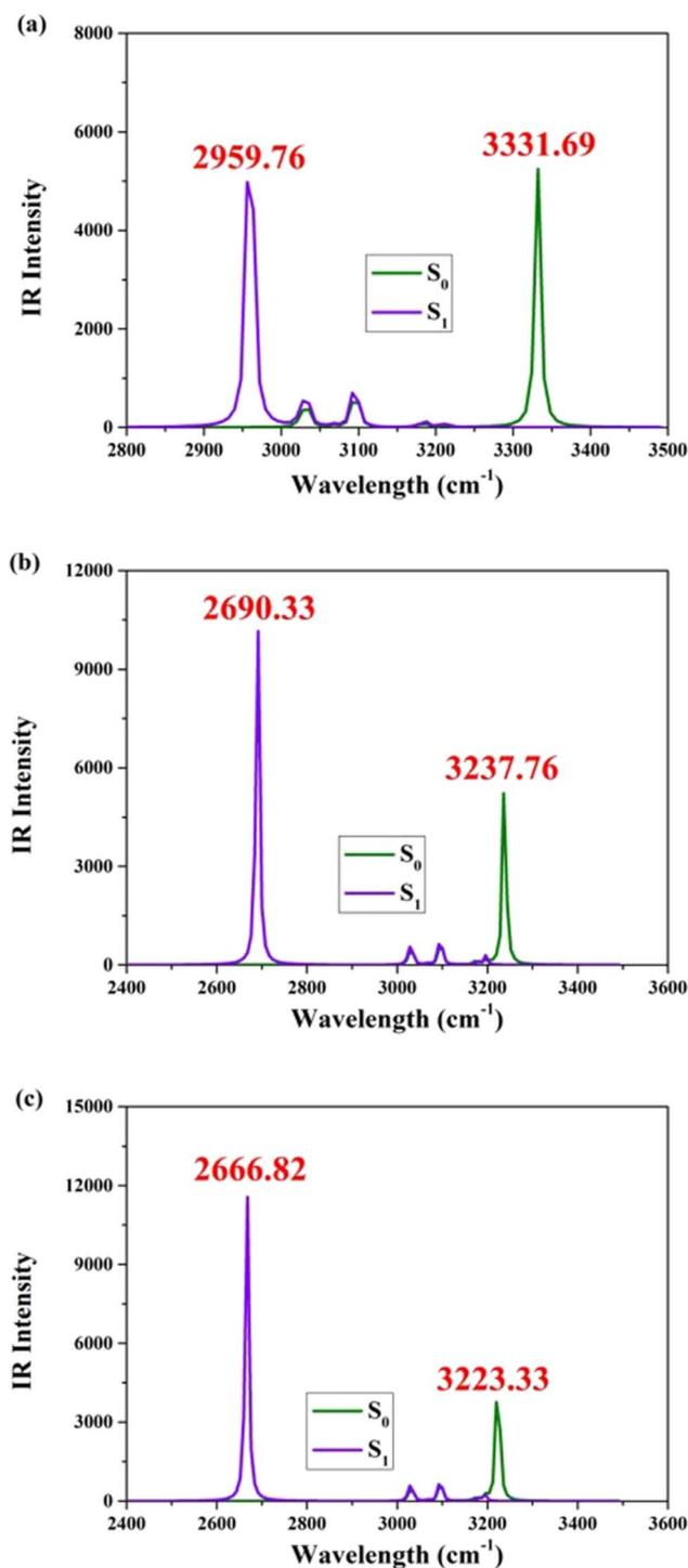
Fig. 2 Computational IR vibrational behaviors of synergetic O1–H2 and O4–H5 stretching vibrational mode for (a) BBHQ-OO, (b) BBHQ-SS and (c) BBHQ-SeSe in  $S_0$  and  $S_1$  states.
