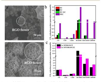
Fig. 10 (a) SEM images of the Cu NP/f-RGO/CF electrode (at different resolutions); (b) CO $_2$  reduction product generation rates on Cu NP/f-RGO/CF electrodes in a Pt-TNT photoanode-driven PEC cell under PC, EC, or PEC conditions. The voltage applied through the cell was 2 V under EC and PEC conditions; (c) CO $_2$  reduction product generation rates on the Cu NP/f-RGO/CF and Cu NP/RGO/CF cathodes in a Pt-TNT photoanode-driven PEC cell.  $^{115}$
