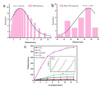
Fig. 6 (a) Diameters of the CNPs and (b) NH<sub>2</sub>-CNPs; (c) photocatalytic reduction products of CO2 on the NH2-CNPs (demonstrating the stability of the NH2-CNPs after 3 repeated uses).88
