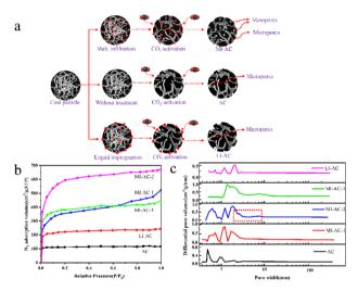
Fig. 3 (a) Schematic depiction of coal-based activated carbon preparation via melt permeation-assisted  $CO_2$  activation; (b)  $N_2$  adsorption/desorption isotherms of the prepared activated carbons; (c) corresponding DFT pore size distributions of the prepared activated carbons.<sup>68</sup>
