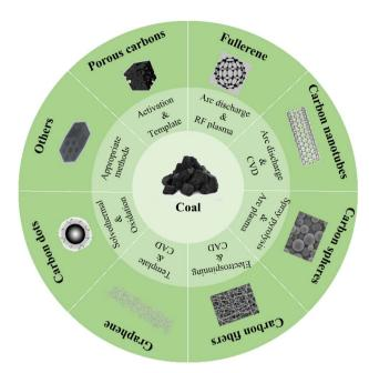
Fig. 2 Different carbon materials derived from coal, highlighting their potential for coal utilization *via* a molecular chemical engineering strategy.<sup>48</sup>
