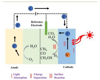
Fig. 9 Schematic diagram of the photoelectric catalysis of  ${\rm CO_2}$  reduction. $^{\rm 110}$
