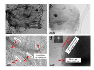
Fig. 4 (a) and (b) Transmission electron microscopy images of 10% FLG samples at different magnifications; (c) and (d) HRTEM images of the FLG film (including an FFT image in the illustration).<sup>82</sup>
