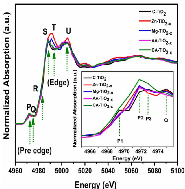
Fig. 3 XANES spectra of C-TiO<sub>2</sub>, Zn-TiO<sub>2-x</sub>, Mg-TiO<sub>2-x</sub>, AA-TiO<sub>2-x</sub> and CA-TiO<sub>2-x</sub> nanocatalysts. The dotted vertical lines highlight the pre edge region (P and Q), and above the edge (R, S, T and U). The inset shows main pre-edge features of all nanomaterials (P1, P2, P3 and Q).
