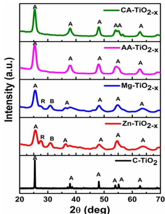
Fig. 1 XRD patterns of C-TiO<sub>2</sub>, Zn-TiO<sub>2-x</sub>, Mg-TiO<sub>2-x</sub>, AA-TiO<sub>2-x</sub> and CA-TiO<sub>2-x</sub> nanocatalysts.
