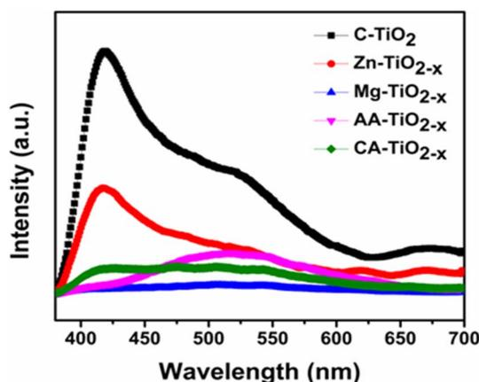
Fig. 7 Steady state photoluminescence (SSPL) plots of the C-TiO<sub>2</sub>, Zn-TiO<sub>2-x</sub>, Mg-TiO<sub>2-x</sub>, AA-TiO<sub>2-x</sub> and CA-TiO<sub>2-x</sub> photocatalysts.
