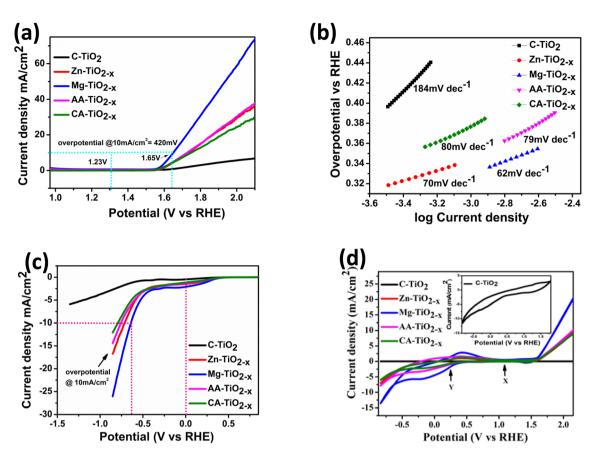
Fig. 8 (a) Linear sweep voltammetric (LSV) data of electrocatalysts for the OER, (b) comparison of Tafel plot for OER of electrocatalysts, (c) linear sweep voltammograms of electrocatalysts for HER and (d) cyclic voltammograms of prepared electrocatalysts and C-TiO<sub>2</sub> (inset).
