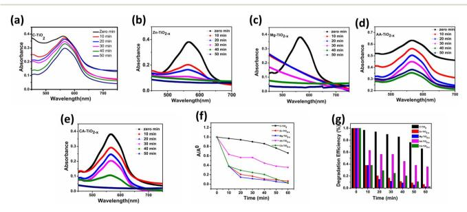
Fig. 11 (a-e) Change in absorbance of RB-866 as a function of irradiation time in the presence of photocatalysts, (f and g) change in concentration of RB-866 dye as a function of irradiation time in the presence of photocatalysts.
