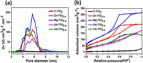
(a) Pore size distribution plots of the nano-catalysts (b)  $N_2$  adsorption-desorption isotherms of all the nanomaterials.
