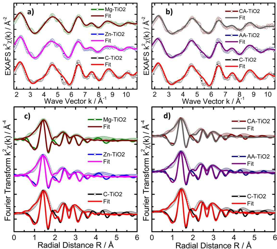
Fig. 4 The  $k^2$ -weighted EXAFS plots (top) and their Fourier transforms (bottom) with best fits at the Ti K-edge for C-TiO<sub>2</sub> and synthesized reduced TiO<sub>2-x</sub>, including Zn-TiO<sub>2-x</sub>, Mg-TiO<sub>2-x</sub> (a and c), AA-TiO<sub>2-x</sub> and CA-TiO<sub>2-x</sub> (b and d), showing the amplitude and the real parts of the Fourier transforms of the data and the fits.
