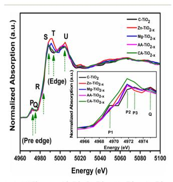
Fig. 3 XANES spectra of  $C-TiO_2$ ,  $Zn-TiO_{2-x}$ ,  $Mg-TiO_{2-x}$ ,  $AA-TiO_{2-x}$  and  $CA-TiO_{2-x}$  nanocatalysts. The dotted vertical lines highlight the pre edge region (P and Q), and above the edge (R, S, T and U). The inset shows main pre-edge features of all nanomaterials (P1, P2, P3 and Q).
