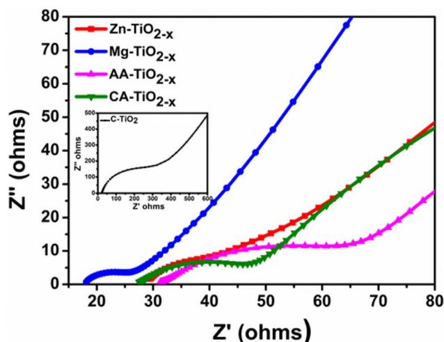
Fig. 9 Nyquist plot of the synthesized electrocatalysts and their comparison with C-TiO<sub>2</sub> (inset).
