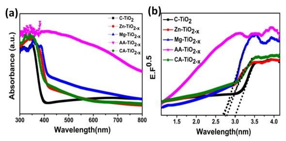
Fig. 6 (a) UV-visible plots of the photocatalysts (b) DRS spectra of different photocatalysts.
