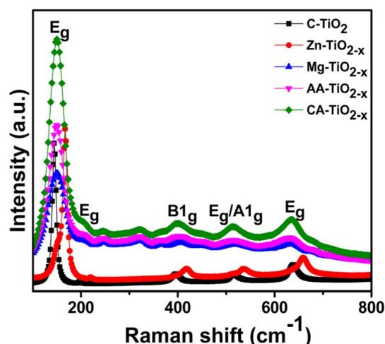
Fig. 2 Raman spectra of C-TiO<sub>2</sub>, Zn-TiO<sub>2-x</sub>, Mg-TiO<sub>2-x</sub>, AA-TiO<sub>2-x</sub> and CA-TiO<sub>2-x</sub> nanocatalysts.
