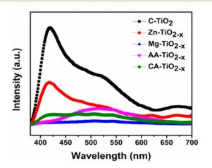
Fig. 7 Steady state photoluminescence (SSPL) plots of the C-TiO $_2$ , Zn-TiO $_2$ - $_x$ , Mg-TiO $_2$ - $_x$ , AA-TiO $_2$ - $_x$  and CA-TiO $_2$ - $_x$  photocatalysts.
