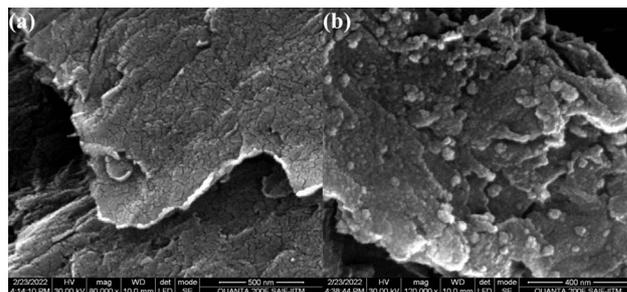
Fig. 7 FE-SEM images: (a) GO and (b) GO-Te-Pd(0).
