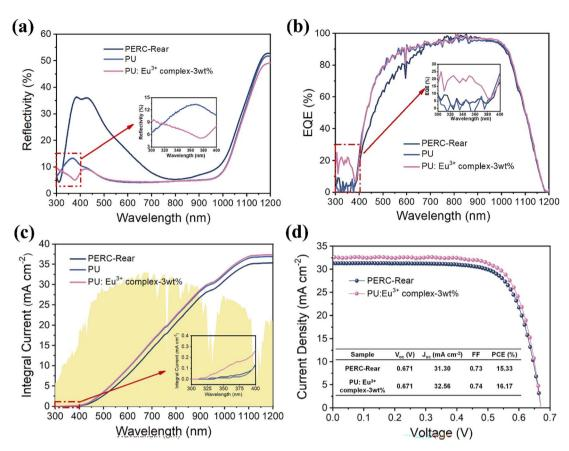
Fig. 6 (a) Reflectance spectra, (b) EQE spectra and (c) integral current density spectra of bi-PERC solar cells coated with PU film and PU:Eu $^{3+}$  complex-3 wt% film on the backside (the inset shows the magnified spectra of 300–400 nm band), (d) J-V curves of bi-PERC solar cells with PU:Eu $^{3+}$  complex-3 wt% film on the backside.
