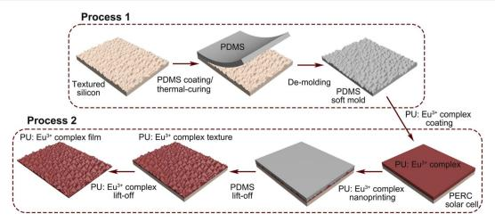
Fig. 2 Schematic illustration of transfer random positive-pyramidal morphology to PU:Eu<sup>3+</sup> complex film.
