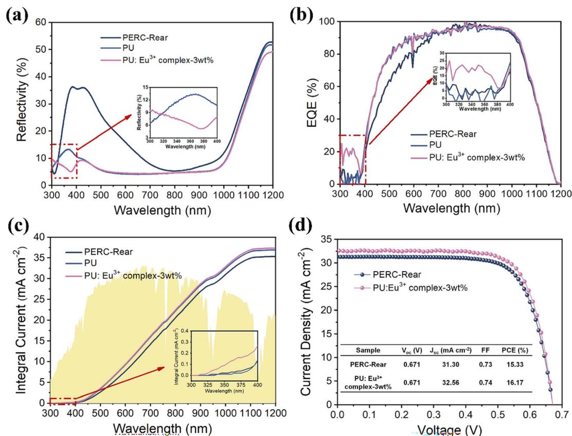
Fig. 6 (a) Reflectance spectra, (b) EQE spectra and (c) integral current density spectra of bi-PERC solar cells coated with PU film and PU:Eu<sup>3+</sup> complex-3 wt% film on the backside (the inset shows the magnified spectra of 300–400 nm band), (d)  $J$ - $V$  curves of bi-PERC solar cells with PU:Eu<sup>3+</sup> complex-3 wt% film on the backside.
