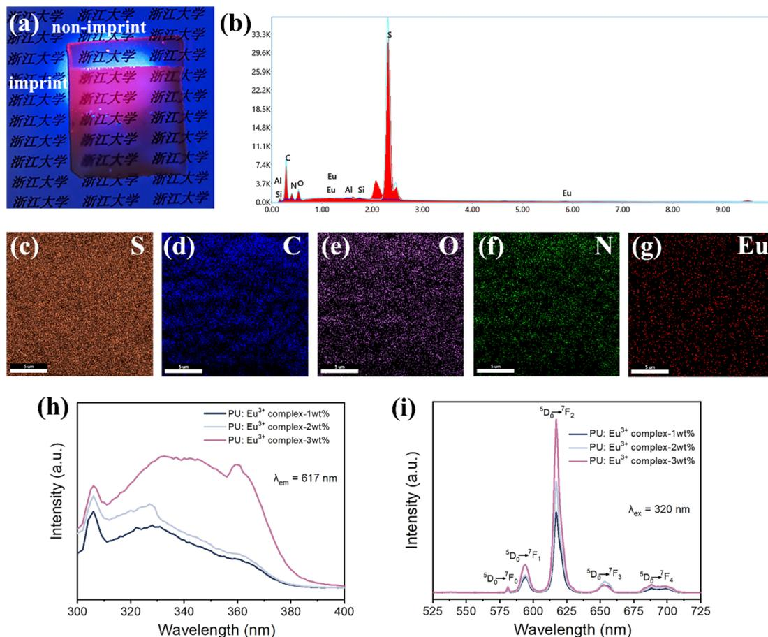
Fig. 4 (a) Digital photography of PU:Eu<sup>3+</sup> complex-3 wt% film when exposed to UV light at 365 nm, (b) EDX spectrum, (c) S, (d) C, (e) O, (f) N and (g) Eu element distribution map of the surface of PU:Eu<sup>3+</sup> complex-3 wt% film, the photoluminescence (h) excitation and (i) emission spectra of PU:Eu<sup>3+</sup> complex films (Eu<sup>3+</sup> complex content: 1, 2, and 3 wt%).
