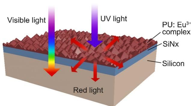
Fig. 5 Schematic illustration of down-conversion mechanism of PU:Eu<sup>3+</sup> complex film coated silicon solar cell.
