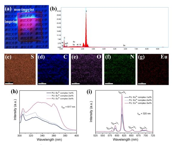
Fig. 4 (a) Digital photography of PU: $Eu^{3+}$  complex-3 wt% film when exposed to UV light at 365 nm, (b) EDX spectrum, (c) S, (d) C, (e) O, (f) N and (g) Eu element distribution map of the surface of PU: $Eu^{3+}$  complex-3 wt% film, the photoluminescence (h) excitation and (i) emission spectra of PU: $Eu^{3+}$  complex films ( $Eu^{3+}$  complex content: 1, 2, and 3 wt%).
