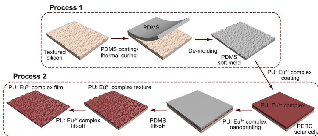
Fig. 2 Schematic illustration of transfer random positive-pyramidal morphology to PU:Eu<sup>3+</sup> complex film.
