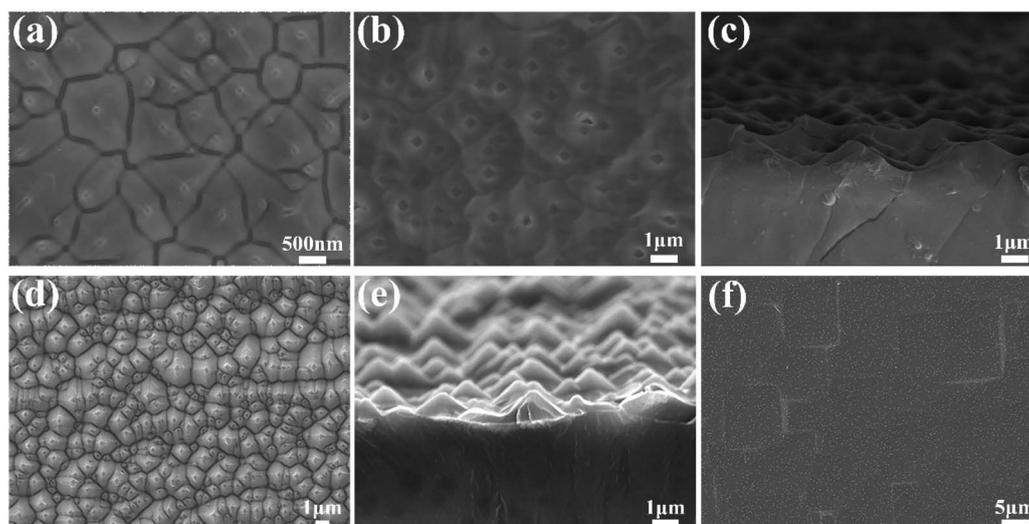
Fig. 3 SEM image of (a) the surface of textured silicon master template, (b) the surface of PDMS soft template, (c) the cross-section of the PDMS soft template, (d) the surface of PU:Eu<sup>3+</sup> complex-3 wt% film, (e) the cross-section of PU:Eu<sup>3+</sup> complex-3 wt% film and (f) the backside of bi-PERC solar cell.
