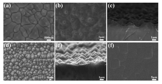
Fig. 3 SEM image of (a) the surface of textured silicon master template, (b) the surface of PDMS soft template, (c) the cross-section of the PDMS soft template, (d) the surface of PU:Eu<sup>3+</sup> complex-3 wt% film, (e) the cross-section of PU:Eu<sup>3+</sup> complex-3 wt% film and (f) the backside of bi-PREC solar cell.
