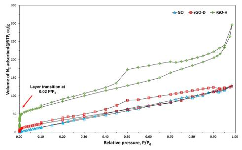
Fig. 4 N<sub>2</sub> adsorption-desorption isotherm of GO, rGO-D, and rGO-H.
