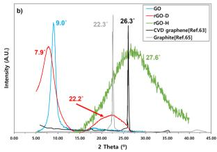
Fig. 5 (a) Raman spectra of GO, rGO-D, rGO-H, and graphite; (b) XRD analysis of GO, rGO-D, rGO-H, and comparison with graphite, and CVD of graphene for reference.
