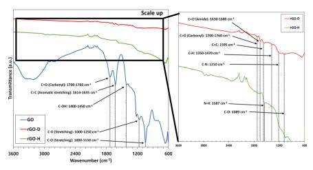
Fig. 3 FT-IR spectra of GO, rGO-D, and rGO-H.
