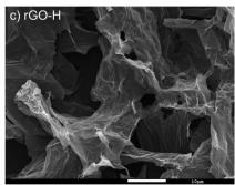
Fig. 1 FE-SEM image of the prepared graphene materials. (a) GO; (b) rGO-D; (c) rGO-H.
