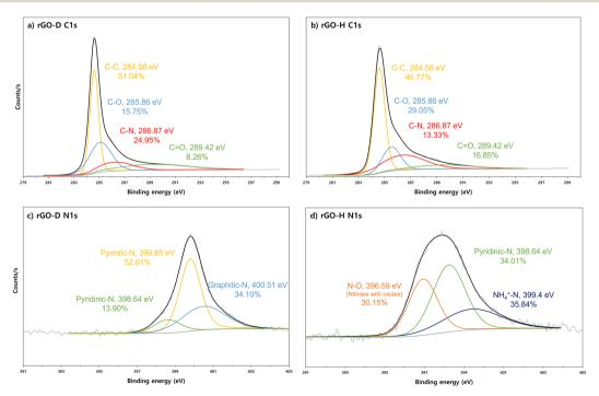
Fig. 2 C 1s and N 1s spectra of rGO-D and rGO-H. (a) C 1s of rGO-D; (b) C 1s of rGO-H; (c) N 1s of rGO-D; (d) N 1s of rGO-H.
