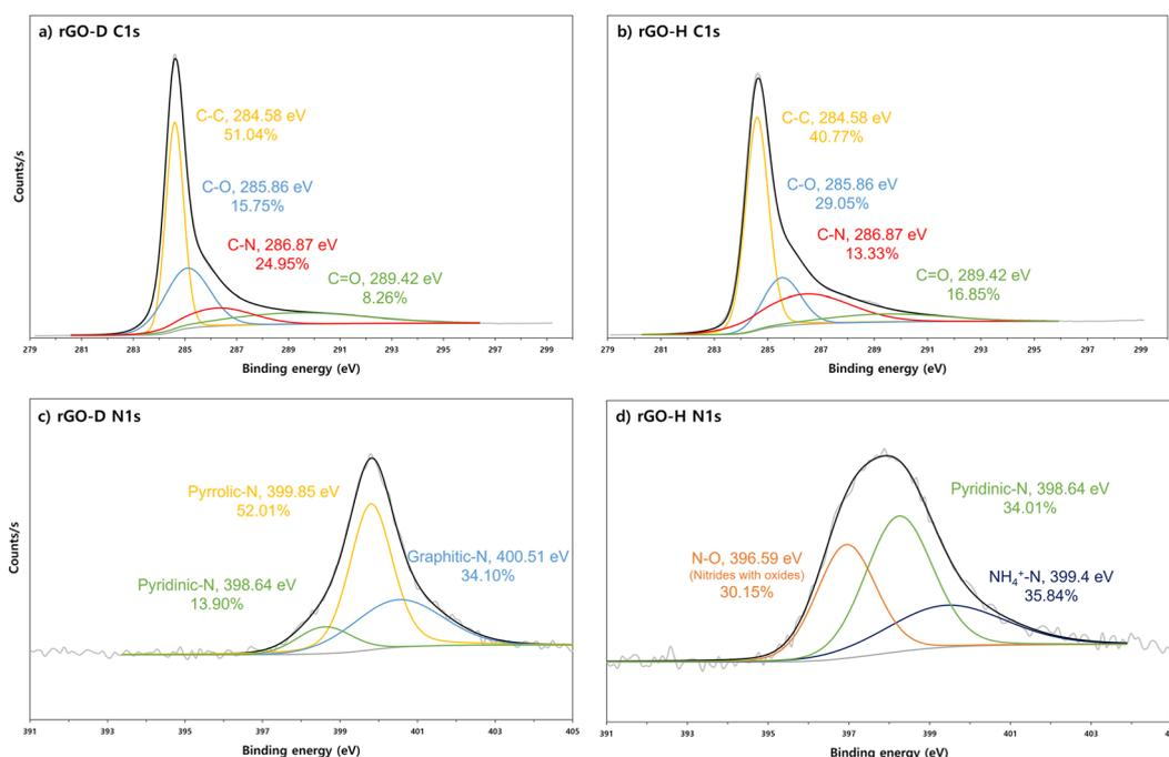
**Fig. 2** C 1s and N 1s spectra of rGO-D and rGO-H. (a) C 1s of rGO-D; (b) C 1s of rGO-H; (c) N 1s of rGO-D; (d) N 1s of rGO-H.
