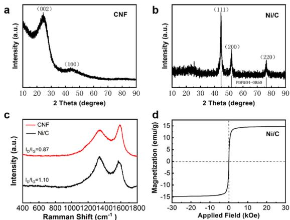
Fig. 4 XRD image of carbon nanofibers (a); XRD image (b), Raman spectra (c) and hysteresis loops (d) of Ni/C nanofibers.
