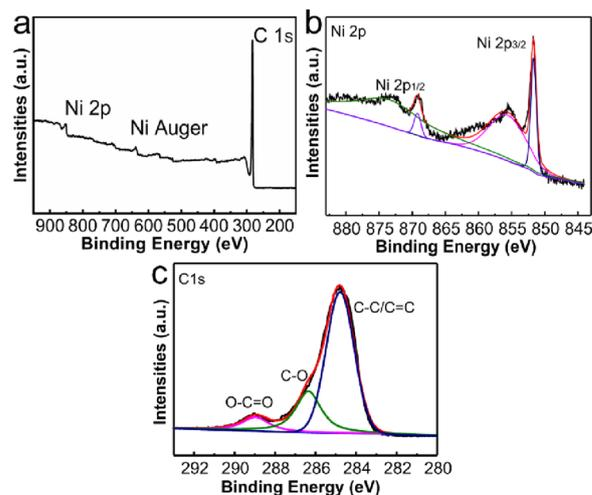
Fig. 5 XPS spectra of Ni/C nanofibers: the survey scans (a), Ni 2p spectrum (b) and C 1s spectrum (c) of Ni/C nanofibers.
