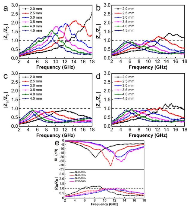
Fig. 9 The values of  $|Z_{in}/Z_0|$  as a function of frequency for various thicknesses for Ni/C-30% (a), Ni/C-50% (b), Ni/C-70% (c), and CNF-50% (d). Reflection loss and impedance matching for optimal microwave absorption performance over all samples (e).
