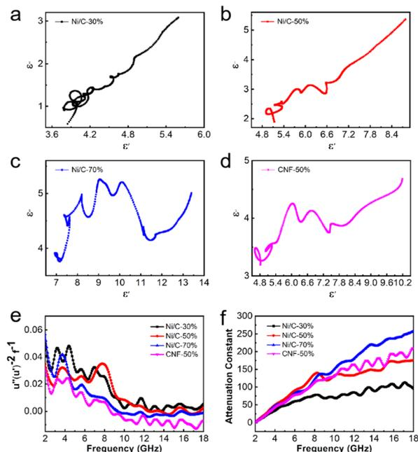
Fig. 8 Curves of  $\epsilon'$  versus  $\epsilon''$  (Cole–Cole semicircles) for Ni/C-30% (a), Ni/C-50% (b), Ni/C-70% (c), and CNF-50% (d). Frequency dependences of  $\mu'' (\mu')^{-2} f^{-1}$  for 30%, 50% and 70% of Ni/C nanofibers (e). Attenuation constant (f) for Ni/C-30%, Ni/C-50%, Ni/C-70%, and CNF-50%.
