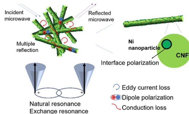
Fig. 10 Microwave absorption mechanism of Ni/C nanofibers.
