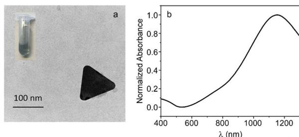
Fig. 1 (a) Transmission electron microscopy (TEM) image showing the triangular shape of the AuNPRs synthesized in the work and digital image showing the green colour of the solution. (b) Normalized absorption spectrum of AuNPRs in phosphate buffer.
