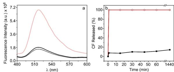
**Fig. 8** (a) Fluorescence emission spectra of CF encapsulated in liposomes coencapsulated with AuNPRs within BioSi@NPs before (black dot) and after (red line) irradiation, and without AuNPRs after irradiation (black line). (b) Release kinetics of CF in % as a function of time (0–1440 min) from TSLs in both absence (black squares) and presence (red circles) of AuNPRs coencapsulated within biomimetic silica nanoprisms.
