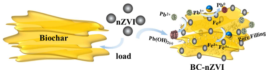
Fig. 12 Proposed a mechanism diagram for the adsorption and reduction of Pb(II) by BC-nZVI.
