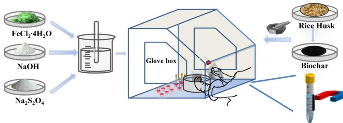
Fig. 1 Schematic diagram of the preparation of BC-nZVI.
