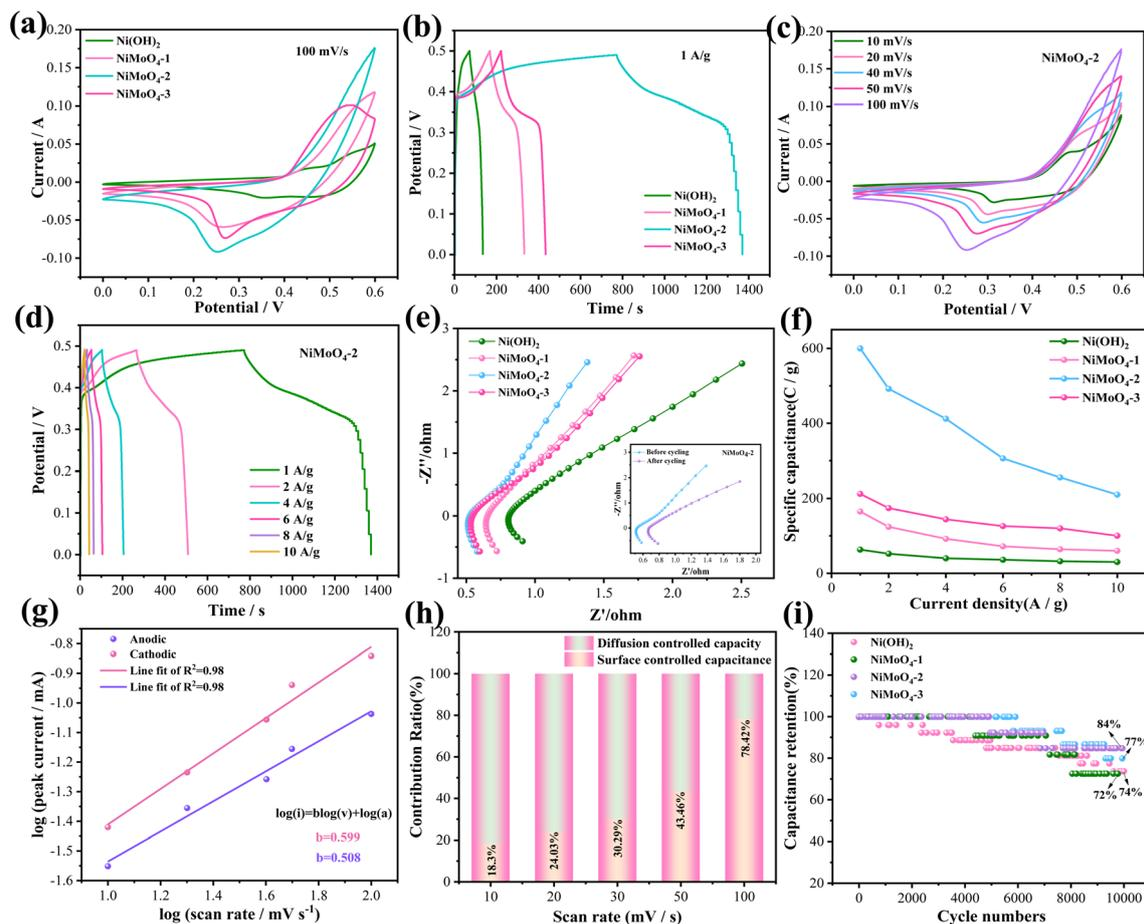
Fig. 3 Electrochemical performance of the electrode materials. (a) CV curves. (b) GCD curves. (c) CV curves of NiMoO<sub>4-2</sub> sample at different scan rates. (d) GCD curves of NiMoO<sub>4-2</sub> sample at different current densities. (e) Nyquist plots. (f) Specific capacitance. (g) *b* value of NiMoO<sub>4-2</sub>. (h) Contribution ratio between surface and diffusion-limited capacities. (i) Cycling performance.
