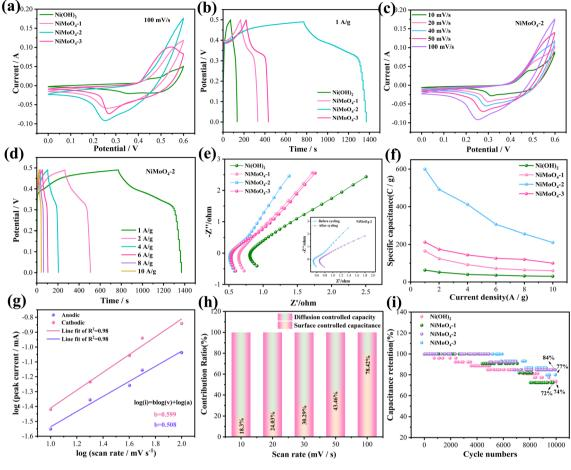
Fig. 3 Electrochemical performance of the electrode materials. (a) CV curves. (b) GCD curves. (c) CV curves of NiMoO<sub>4</sub>-2 sample at different scan rates. (d) GCD curves of NiMoO<sub>4</sub>-2 sample at different current densities. (e) Nyquist plots. (f) Specific capacitance. (g) b value of NiMoO<sub>4</sub>-2. (h) Contribution ratio between surface and diffusion-limited capacities. (i) Cycling performance.
