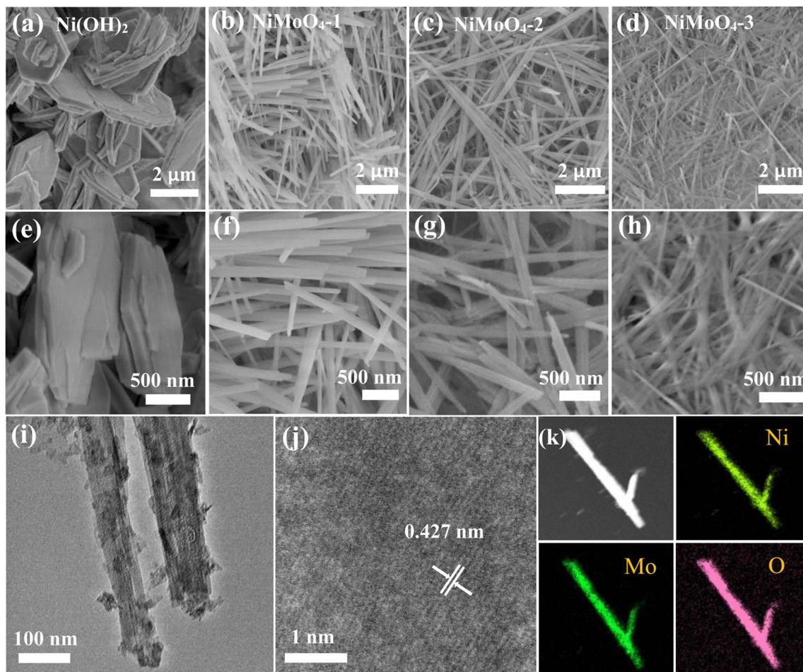
Fig. 2 Morphology characterization. (a) and (e) SEM image of the  $\text{Ni}(\text{OH})_2$  nanosheets. (b) and (f) SEM image of the  $\text{NiMoO}_4\text{-1}$  nanorods. (c) and (g) SEM image of the  $\text{NiMoO}_4\text{-2}$  nanorods. (d) and (h) SEM image of the  $\text{NiMoO}_4\text{-3}$  nanorods. (i) TEM image of  $\text{NiMoO}_4\text{-2}$  samples. (j) HRTEM image. (k) EDS element mappings.
