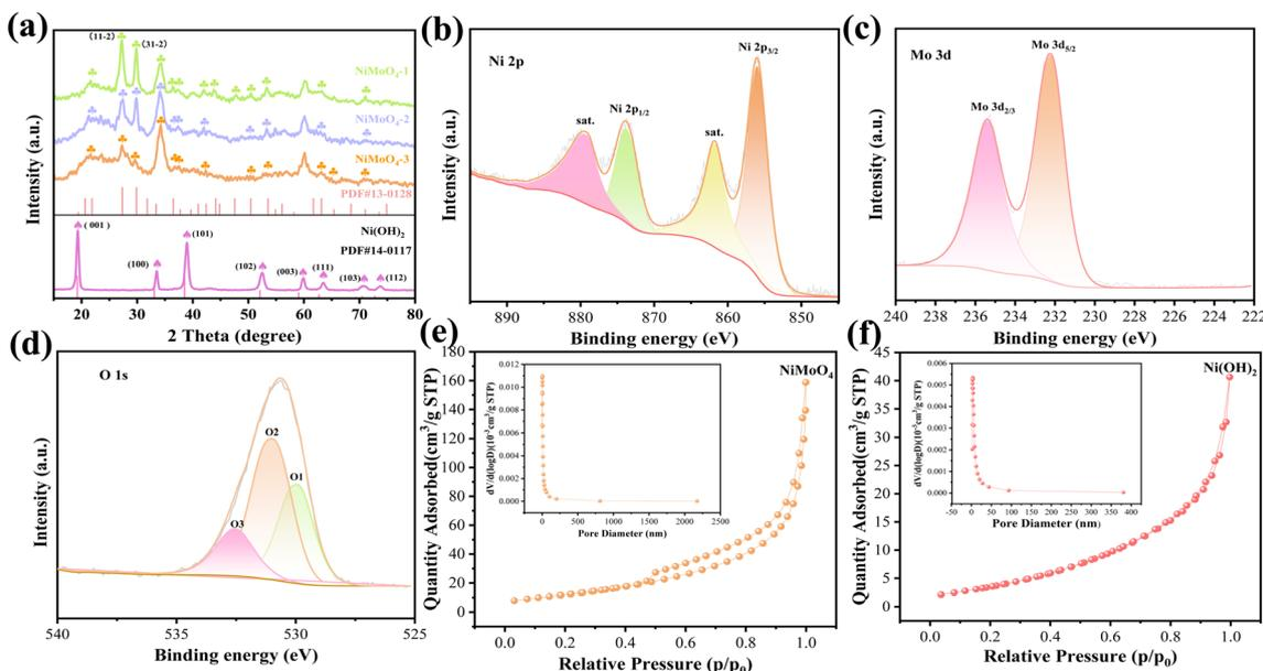
Fig. 1 Structural characterization. (a) XRD patterns. (b)–(d) XPS spectra of the  $\text{NiMoO}_4$ -2 sample. (e) and (f) N<sub>2</sub> adsorption–desorption isotherms (the insets: the pore size distribution curves).
