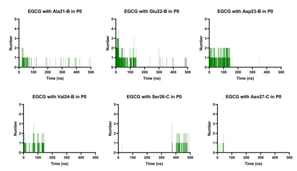
Fig. 9 Prevalent H-bonds in P0 for the EGCG-remodelled oligomer calculated over 500 ns for md1.
