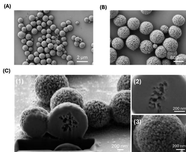
Fig. 3 SEM images at different magnification of porous EG-CaCO<sub>3</sub> MPs: top view ((A), Mag 20.00k $\times$ , EHT 2.00 kV), (B) Mag 50.00k $\times$ , EHT 2.00 kV), cross-section ((C1), Mag 80.00k $\times$ , EHT 2.00 kV, (C2), Mag 250.00k $\times$ , EHT 2.00 kV), porous surface ((C3), 80.00k $\times$ , EHT 2.00 kV).
