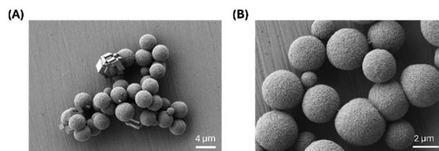
Fig. 1 SEM images of SF-CaCO<sub>3</sub> MCs without L-T4 at low magnification ((A), Mag 7.63k×, EHT 1.00 kV) and high magnification ((B), Mag 20.00k×, EHT 1.00 kV).
