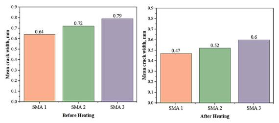
Fig. 13 Variation of crack width for different SMAs.
