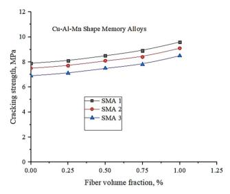
Fig. 11 Variation of cracking strength with fibre volume fraction of Cu–Al–Mn SMA alloys.
