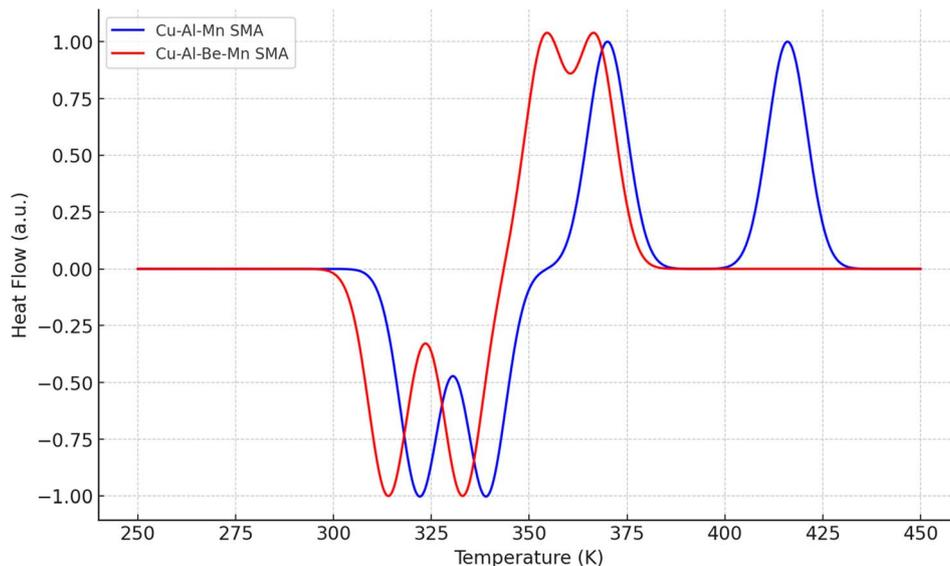
Fig. 15 DSC graph of Cu–Al–Mn and Cu–Al–Be–Mn SMA's.
