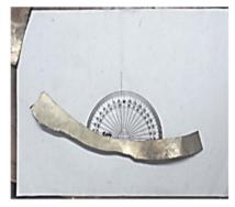
Spring back position **Heating position Deformation Position**
