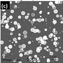
Fig. 17 SE micrograph of microstructural evolution at (a) low, (b) medium and (c) high temperature of Cu-Al-Be-Mn based SMA.
