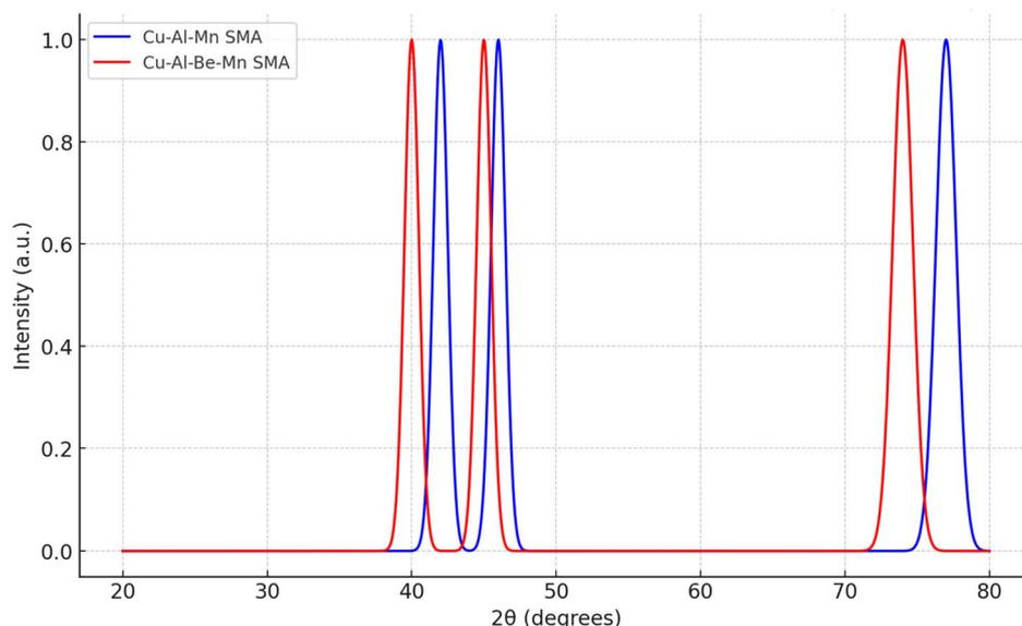
Fig. 14 XRD graph of Cu–Al–Mn and Cu–Al–Be–Mn SMA's.
