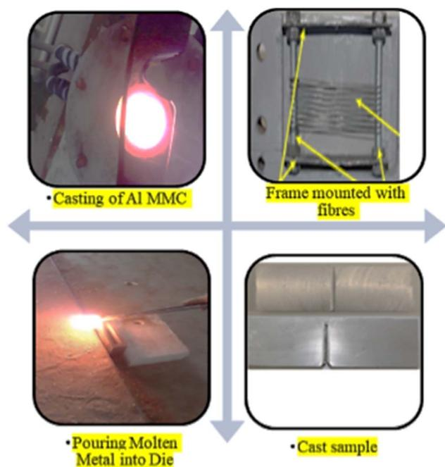
Fig. 4 Preparation of Al metal matrix composites (MMCs).
