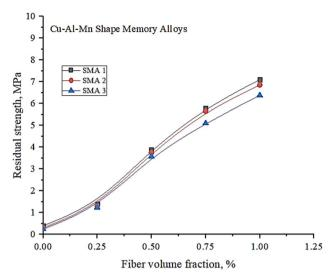
Fig. 7 Variation of residual strength with fibre volume fraction of Cu–Al–Mn SMA alloys.
