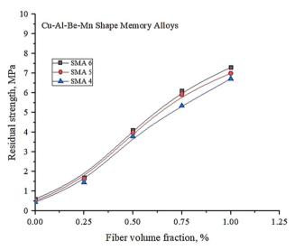
Fig. 8 Variation of residual strength with fibre volume fraction of Cu–Al–Be–Mn SMA alloys.
