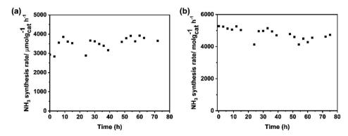
Fig. 11 Ammonia synthesis rate over (a) 1Ba-4 wt% Ru/2.0BaNb and (b) 2Cs-4 wt% Ru/2.0BaNb as a function of time on steam. Reaction conditions: 100.0 mg of catalyst, 60 mL (STP) min<sup>-1</sup> of synthesis gas  $(3H_2 + N_2)$  at 673 K and 0.1 MPa.
