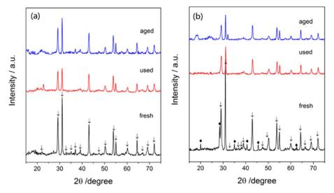
Fig. 12 XRD images of (a)  $1Ba-4Ru/Ba_5Nb_4O_{15}$  and (b)  $2Cs-4Ru/Ba_5Nb_4O_{15}$  measured at different phases: as-prepared (fresh), after activity tests (used), and after stability tests (aged). Reaction conditions: 100.0 mg of catalyst, and 60 mL (STP) min<sup>-1</sup> of synthesis gas ( $3H_2 + N_2$ ), at 0.1 MPa.
