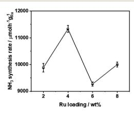
Fig. 5 Ammonia synthesis rate of different Ru loadings on Ba<sub>5</sub>Nb<sub>4</sub>O<sub>15</sub>. Reaction conditions: prior to activity tests, the catalysts (100.0 mg) were reduced in H<sub>2</sub> flow of 15 mL min<sup>-1</sup> at 573 K for 3 h; the activities were tested in 60 mL (STP) min<sup>-1</sup> of synthesis gas  $(3H_2 + N_2, 99.999\%)$ at 673 K and 0.1 MPa.
