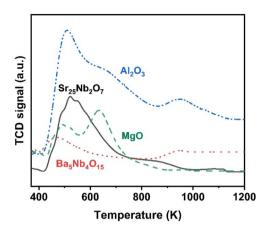
Fig. 10 NH<sub>3</sub>-TPD profiles obtained over  $Ba_5Nb_4O_{15}$  (2.0 BaNb),  $Sr_2Nb_2O_7$  (2.0 SrNb),  $\gamma$ -Al $_2O_3$ , and MgO. Samples (100.0 mg) were exposed to 5 vol% NH $_3$  in N $_2$  flow (10 mL min $^{-1}$ ) at 373 K for 30 min, and desorptions were performed from 373 to 1073 K at 10 K min $^{-1}$  in N $_2$  carrier gas flow (15 mL min $^{-1}$ ).
