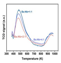
Fig. 2 Ammonia TPD profiles obtained over different molar ratios of Ba/Nb. Samples (100.0 mg) were exposed to 5 vol% NH<sub>3</sub> in N<sub>2</sub> flow (10 mL min<sup>-1</sup>) at 373 K for 30 min, and desorptions were performed from 373 to 1073 K at 10 K min<sup>-1</sup> in N<sub>2</sub> carrier gas flow (15 mL).
