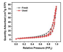
Fig. 6 Adsorption/desorption isotherm of fresh and used 4% Ru/ Ba<sub>5</sub>Nb<sub>4</sub>O<sub>15</sub>.
