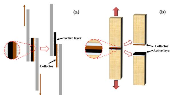
Fig. 3 Schematic diagram of the interfacial strength experiment: (a) shear and (b) lap.
