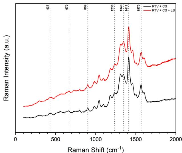
Fig. 9 Raman spectra for the meshes RTV + CS and RTV + CS + LS.
