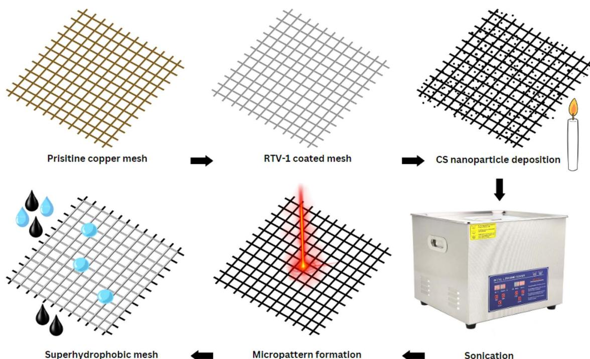
Fig. 1 Stepwise procedure for fabricating superhydrophobic mesh.
