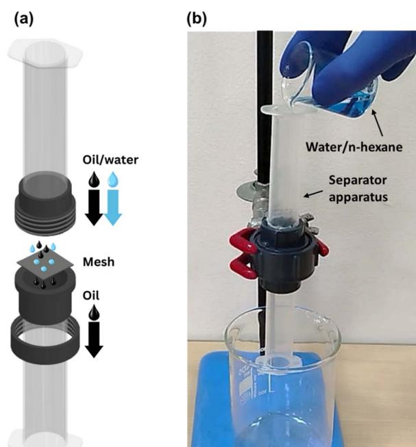
Fig. 3 (a) Exploded-view diagram and (b) actual photograph of the gravity-driven oil/water separator column employed in this study.
