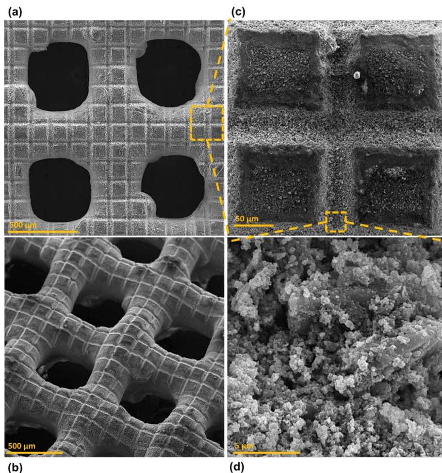
Fig. 6 SEM image of femtosecond laser structured copper mesh coated with CS using RTV-1 as binder (RTV + CS + LS) with plane (a) parallel and (b) tilted 40° relative to the sample stage. (c) is a zoomed in view of the segment highlighted in (a), and (d) is a zoomed in view of the segment highlighted in (c).
