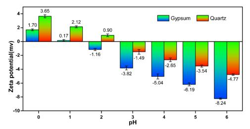
Fig. 7 Zeta potential analysis results of gypsum and guartz.
