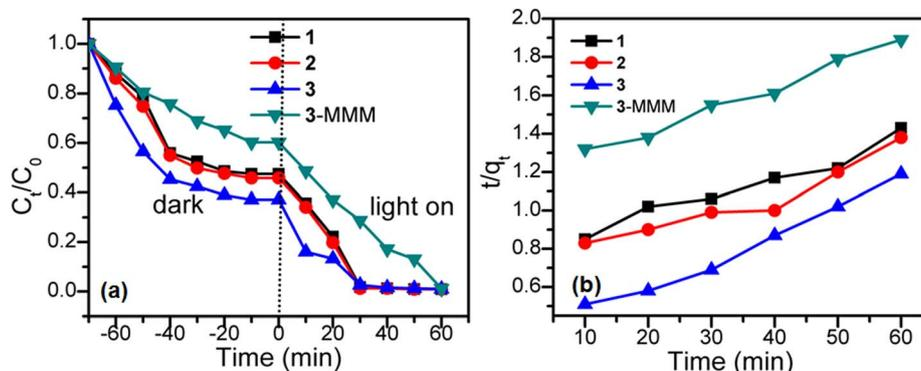
Fig. 6 (a) Adsorption and photocatalytic degradation of the methyl blue solution ( $80 \text{ mg L}^{-1}$ , 20 mL) by 1, 2, 3 and 3-MMM. (b) Pseudo-second-order adsorption kinetic fitting of 1, 2, 3 and 3-MMM in the MB solution.
