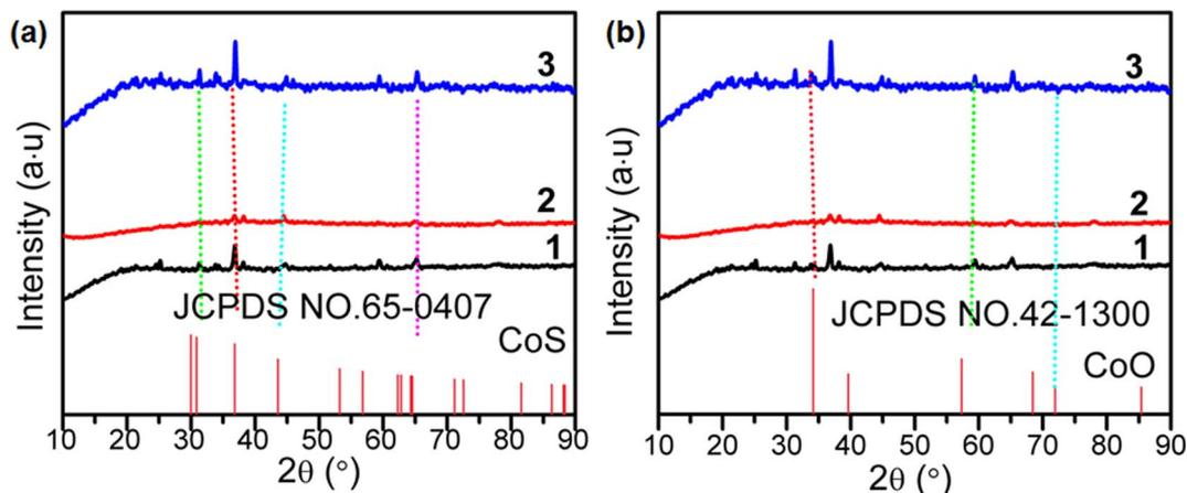
Fig. 1 (a) XRD patterns of CoS and 1–3. (b) XRD patterns of CoO and 1–3.
