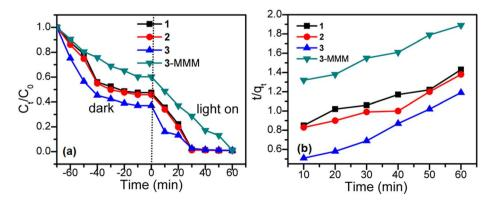
Fig. 6 (a) Adsorption and photocatalytic degradation of the methyl blue solution (80 mg  $L^{-1}$ , 20 mL) by 1, 2, 3 and 3-MMM. (b) Pseudo-second-order adsorption kinetic fitting of 1, 2, 3 and 3-MMM in the MB solution.
