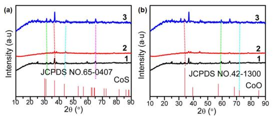
Fig. 1 (a) XRD patterns of CoS and 1-3. (b) XRD patterns of CoO and 1-3.
