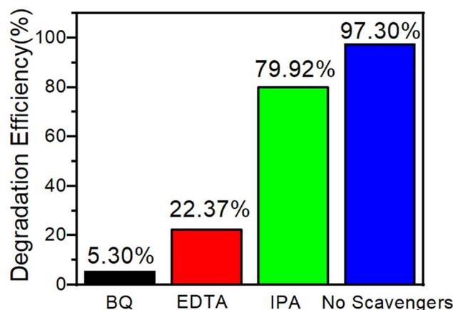
Fig. 9 Trapping experiment of active species during the photocatalytic degradation of MB over 3 under light irradiation.
