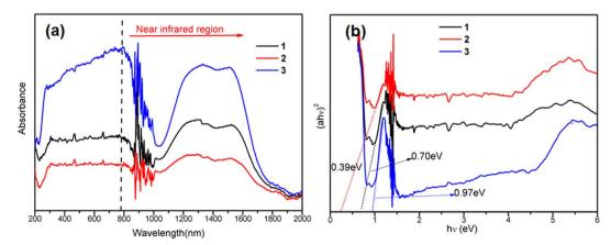
Fig. 4 (a) Solid-state UV-vis-NIR absorption spectra of 1, 2 and 3. (b) Plots of  $(\alpha hv)^2$  versus photon energy (hv) for the bandgap energies of 1, 2 and 3.
