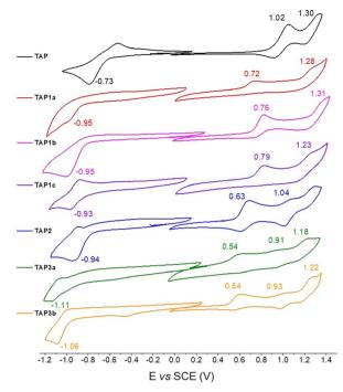
Fig. 3 Cyclic voltammograms of TAP1-3 recorded in DCM ( $10^{-3}$  M) in the presence of tetra-n-butylammonium hexafluorophosphate as supporting electrolyte ( $10^{-1}$  M), with a scan rate of 100 mV s<sup>-1</sup>.
