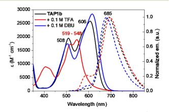
Fig. 6 Electronic absorption (solid lines,  $c = 1.15 \times 10^{-5}$  M) and normalized emission (dashed lines) spectra of TAP1b in DCM ( $\lambda_{ex} = 510$ nm), DCM + TFA ( $\lambda_{ex} = 510$  nm) and DCM + DBU ( $\lambda_{ex} = 565$  nm).
