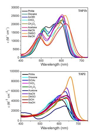
Fig. 5 Electronic absorption solvatochromism of TAP1b and TAP2 (c =  $1.15 \times 10^{-5}$  M and  $1.3 \times 10^{-5}$  M respectively)
