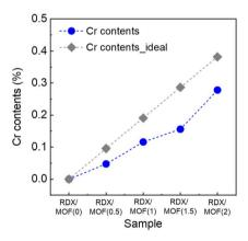
Fig. 3 Cr component in RDX ink obtained through ICP analysis and theoretically calculated value.
