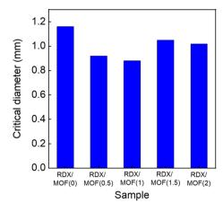
Fig. 7 Results of detonation test of RDX/MOF composites.
