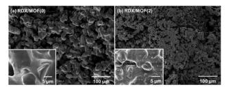
Fig. 4 FESEM images of RDX ink pattern of (a) RDX/GAP and (b) RDX/GAP/MOFs.
