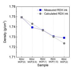
Fig. 5 Density of RDX ink measured by gas pycnometer.
