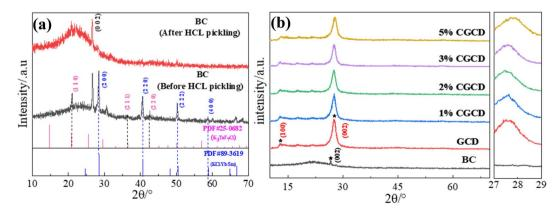
Fig. 2 XRD spectra of different samples. (a) XRD comparison of wheat straw biochar before and after acid leaching; (b) XRD patterns of different samples.
