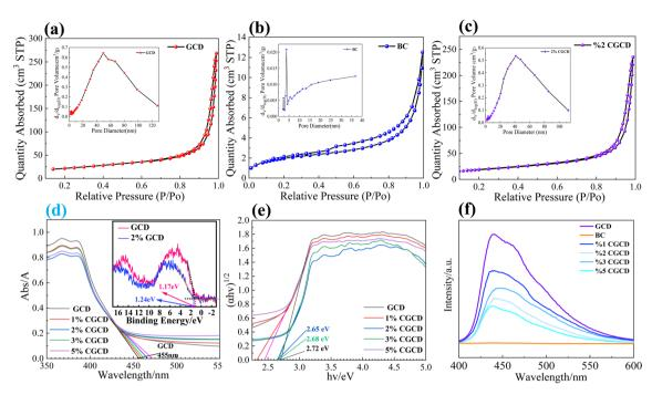
Fig. 6 N₂ isothermal adsorption—desorption curves and pore size distribution of different samples: GCD (a); BC (b); 2% CGCD (c). UV-vis spectra and valence band spectrum of different samples (d); Tauc-curve (e); PL spectra (f).
