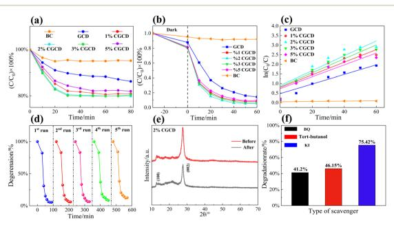
Fig. 7 (a) Adsorption experimental plots of different samples; (b) degradation rate of different photocatalyst samples; (c) fitting diagram of degradation kinetics for different samples; (d) cyclic degradation rate of 2% CGCD with time; (e) XRD patterns of 2% CGCD before and after circulation experiment; (f) pattern of free radical trapping experiment.
