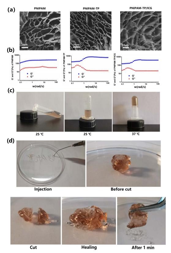
Fig. 2 Dynamic functions, microstructure and rheological characteristics of hydrogels. (a) Scanning electron microscopy images of PNIPAM, PNIPAM-TP, and PNIPAM-TP/ICG hydrogels. (b) Storage modulus (G') and loss modulus (G'') of PNIPAM, PNIPAM-TP, and PNIPAM-TP, and PNIPAM-TP/ICG hydrogels as a function of frequency. (c) Fluidity and (d) injectability of PNIPAM-TP/ICG hydrogel materials at room temperature and in a 37 °C environment.
