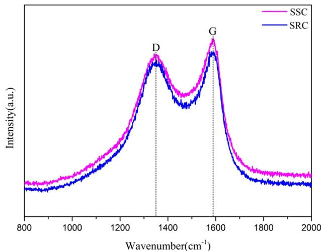
Fig. 4 Raman spectra of SSC and SRC.
