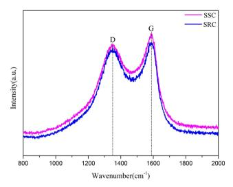
Fig. 4 Raman spectra of SSC and SRC.
