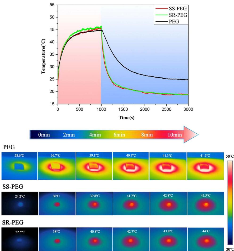
Fig. 10 (a) Temperature curves of PEG, SS-PEG and SR-PEG with time under xenon lamp; (b) infrared thermal images of PEG, SS-PEG and SR-PEG during heating.
