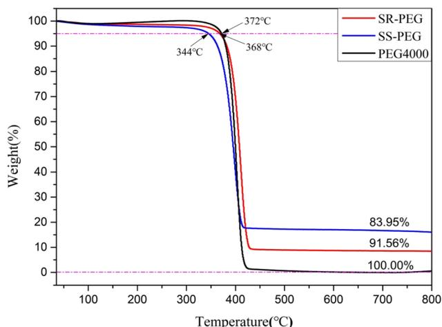
Fig. 9 TGA curves of PEG4000, SS-PEG and SR-PEG.
