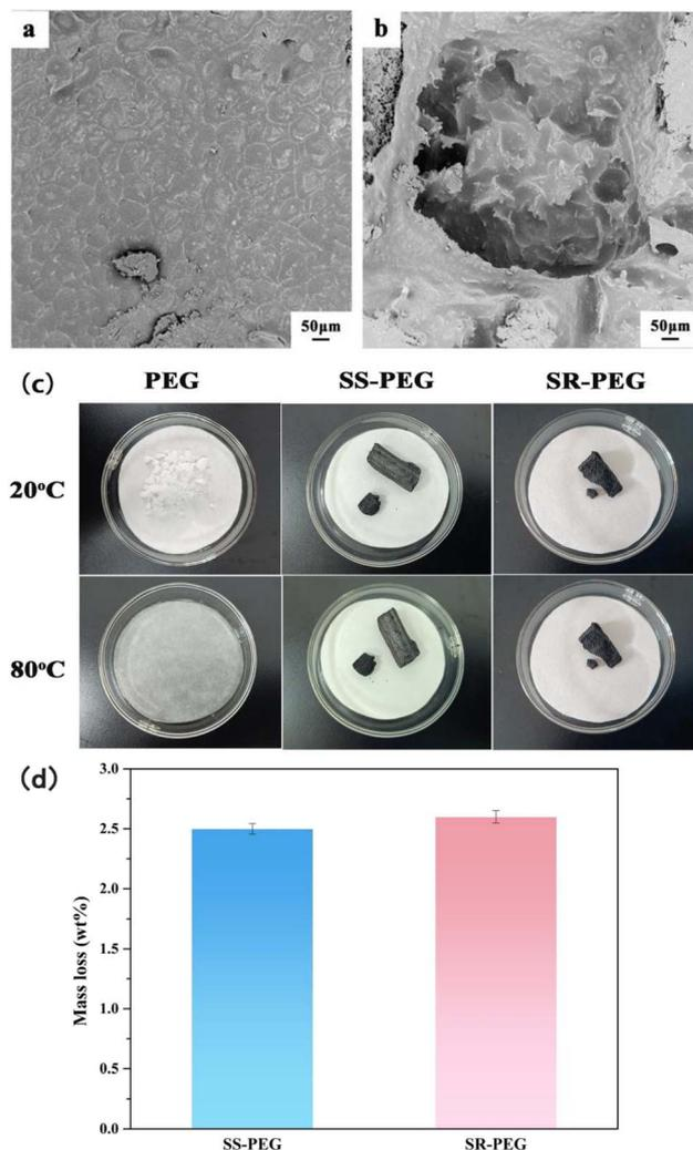
Fig. 5 SEM images of shape-stabilized phase change materials: (a) SS-PEG and (b) SR-PEG; (c) leakage macroscopic morphology of PEG, SS-PEG and SR-PEG under  $80\text{ }^\circ\text{C}$  for 30 min; (d) the leakage rate of SS-PEG and SR-PEG after 100 thermal cycles.
