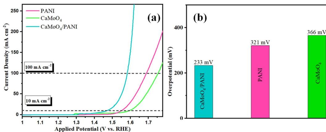
Fig. 6 (a) Polarization curves from the LSV measurements with PANI,  $\text{CaMoO}_4$ , and  $\text{CaMoO}_4/\text{PANI}$ . (b) Bar diagram of the overpotential at  $10 \text{ mA cm}^{-2}$  current density.
