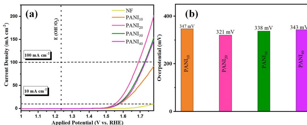
Fig. 5 (a) Polarization curves obtained from the LSV measurements with PANI<sub>10</sub>, PANI<sub>20</sub>, PANI<sub>30</sub>, PANI<sub>40</sub> and NF and (b) comparative representation of the overpotential at current density 10 mA cm<sup>-2</sup>.
