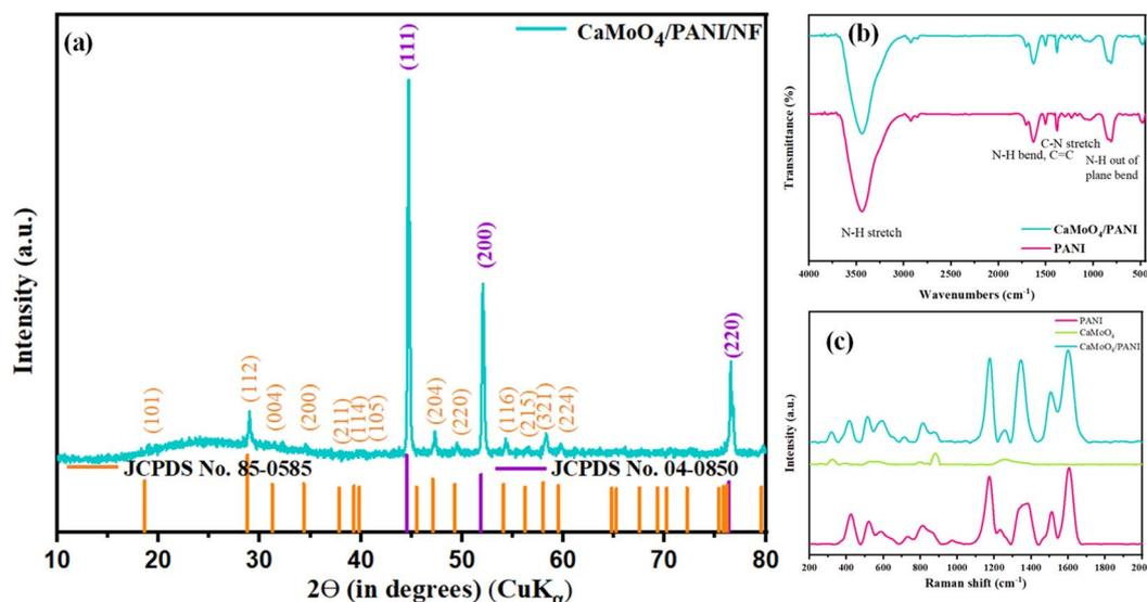
Fig. 1 (a) XRD pattern, (b) FT-IR spectra, and (c) Raman spectra of the synthesized CaMoO<sub>4</sub>, PANI, and CaMoO<sub>4</sub>/PANI catalyst samples.
