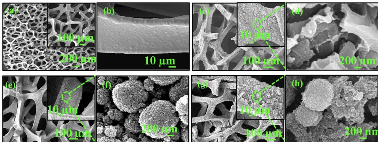
Fig. 2 FESEM images at different magnifications of (a) and (b) bare NF, (c) and (d) PANI, (e) and (f)  $\text{CaMoO}_4$ , and (g) and (h)  $\text{CaMoO}_4/\text{PANI}$ .
