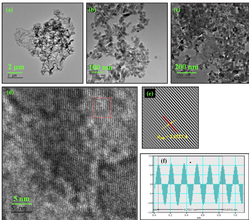
Fig. 3 TEM images of (a) PANI, (b)  $\text{CaMoO}_4$ , (c)  $\text{CaMoO}_4/\text{PANI}$ , (d) HRTEM of  $\text{CaMoO}_4/\text{PANI}$ , (e) IFFT and (f) profile of IFFT  $\text{CaMoO}_4/\text{PANI}$ .
