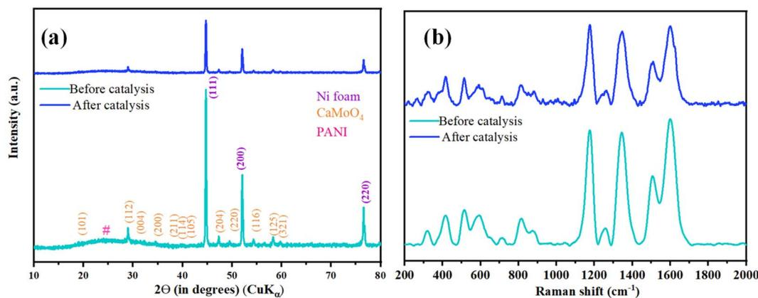
Fig. 10 Before and after catalysis characterization of CaMoO<sub>4</sub>/PANI (a) PXRD pattern and (b) Raman spectra.
