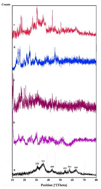
Fig. 3 XRD patterns of  $Fe_3O_4/pectin$  (a), Co-MOF (b), (Co/Cu)MOF (c), Cu-MOF (d),  $Fe_3O_4/pectin/(Co/Cu)MOF$  (e).
