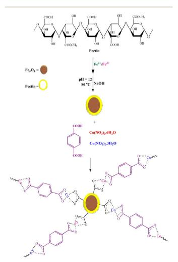
Fig. 1 Preparation of Fe<sub>3</sub>O<sub>4</sub>/pectin/(Co/Cu)MOF nanocomposite.
