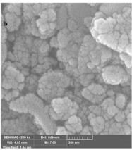
FT-IR spectrum (a), and SEM image (b) of recycled Fe<sub>3</sub>O<sub>4</sub>/pectin/(Co-Cu)MOF.
