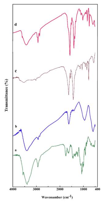
Fig. 2 FT-IR spectra of pectin (a),  $Fe_3O_4/pectin$  (b), (Co/Cu)MOF (c) and  $Fe_3O_4/pectin/(Co/Cu)MOF$  (d).
