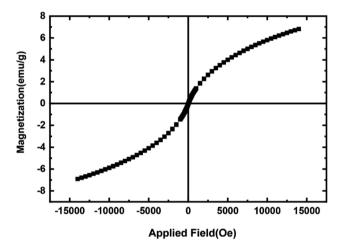
Fig. 7 VSM analysis of Fe<sub>3</sub>O<sub>4</sub>/pectin/(Co/Cu)MOF.
