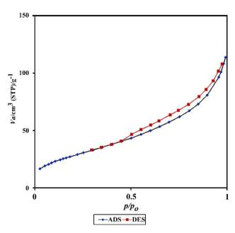
Fig. 8  $N_2$  adsorption—desorption isotherms of  $Fe_3O_4/pectin/(Co/Cu)$  MOF.
