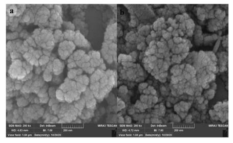
Fig. 4 FE-SEM images of Fe<sub>3</sub>O<sub>4</sub>/pectin/(Co/Cu)MOF
