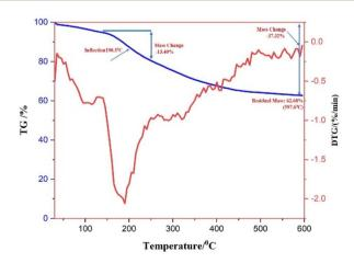
Fig. 9 TGA and DTA pattern of biogenic PdNPs.
