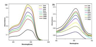
Fig. 17 UV-vis spectra for the catalytic reduction of (a) sunset yellow, (b) indigo carmine in the presence of biogenic PdNPs.
