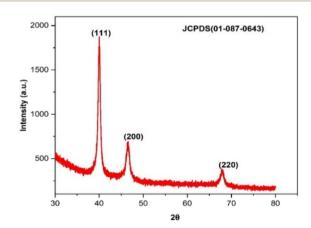
Fig. 8 XRD pattern of biosynthesized palladium nanoparticles.
