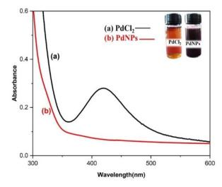
Fig. 4 UV-vis absorption spectra of biogenic PdNPs.
