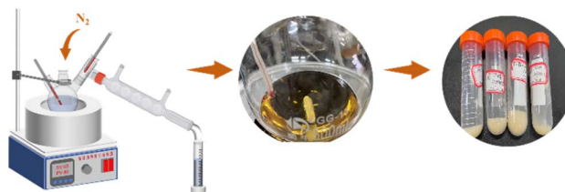
Fig. 2 Copolyester plasticizer preparation process.
