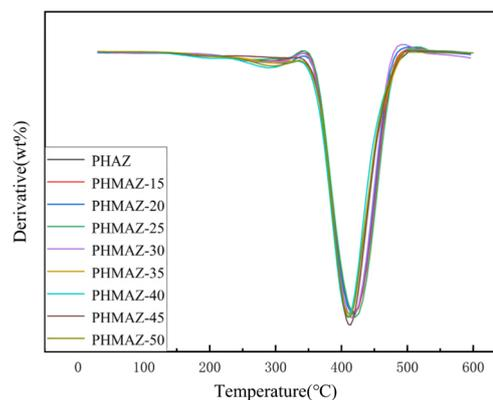
Fig. 9 DTG curves of PHAZ and PHMAZ.
