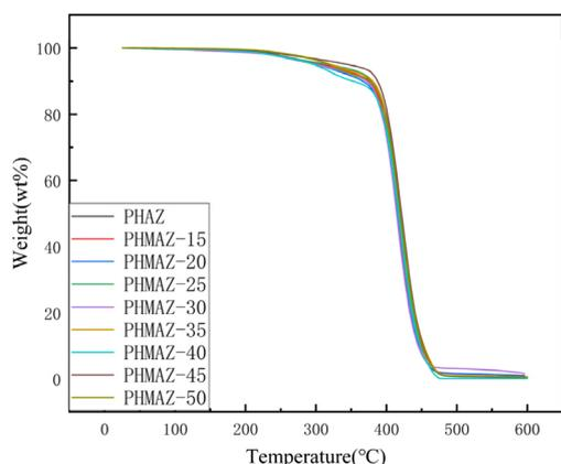
Fig. 8 TG curves of PHAZ and PHMAZ.
