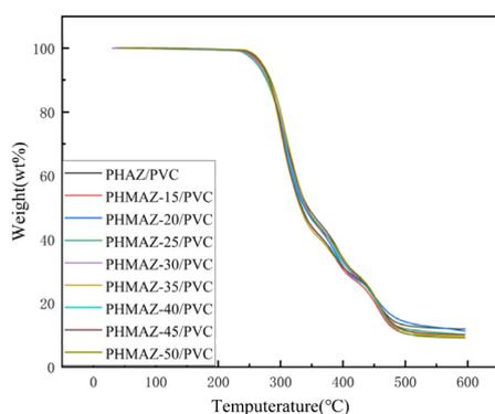
Fig. 12 TG curves of PVC samples plasticized by PHAZ and PHMAZ.
