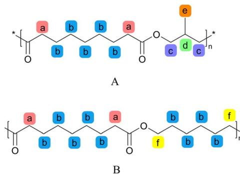
Fig. 5 Two structural units of PHMAZ copolyester.
