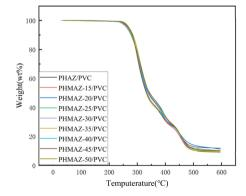
Fig. 12 TG curves of PVC samples plasticized by PHAZ and PHMAZ.
