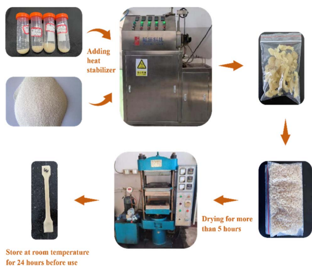
Fig. 3 Preparation of PVC resin splines plasticized with plasticizer.
