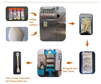
Fig. 3 Preparation of PVC resin splines plasticized with plasticizer.
