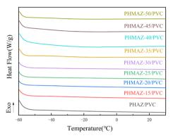
Fig. 10 DSC curves of PHAZ and PHMAZ plasticized PVC samples.
