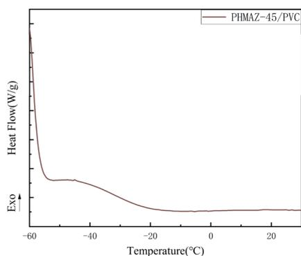
Fig. 11 DSC curve of PHMAZ-45 plasticized PVC sample.
