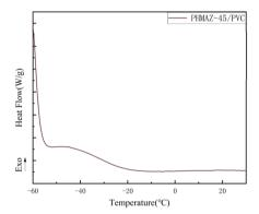
Fig. 11 DSC curve of PHMAZ-45 plasticized PVC sample.
