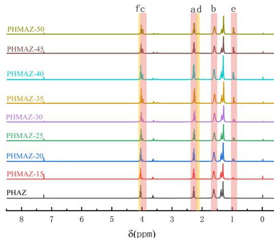
Fig. 6 HNMR spectra of PHAZ and PHMAZ.
