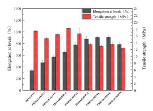
Fig. 14 Mechanical properties graph of PVC samples plasticized with PHAZ and PHMAZ.
