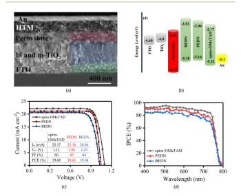
Fig. 4 (a) Diagram of the device structure, SEM cross section of device based on PEDN. (b)Energy level diagram for each layer in PSCs. (c) J-V curves of PSCs and (d) the IPCE plots of PSCs based on PEDN, BEDN, spiro-OMeTAD HTMs.
