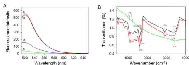
**Fig. 5** (A) Fluorescence emission spectra of the E2 aptamer probe under different conditions: (a) E2 aptamer probe; (b) E2 aptamer probe + E2; (c) BQNP/aptamer probe; (d) BQNP/aptamer probe + E2. The concentrations of BQNP/aptamer probe, E2, and E2 aptamer were 10  $\mu\text{g mL}^{-1}$ , 500  $\text{ng mL}^{-1}$ , and 10 nM, respectively. (B) FTIR spectra of BQNP (red colour), E2 aptamer probe (green colour), and BQNP/aptamer probe (black colour).
