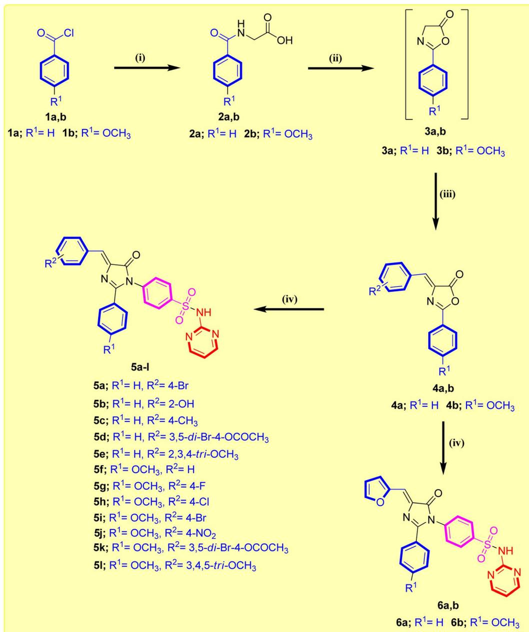
**Scheme 1** Synthesis of imidazolone-sulphonamide-pyrimidine compounds **5a-l** and **6a,b**. Reagents: (i) glycine, aqueous sodium hydroxide, rt, 2 h; (ii) Ac<sub>2</sub>O, 80 °C, 2 h; (iii) respective aryl aldehyde, NaOAc, 80 °C, 2 h; (iv) sulfadiazine, NaOAc, glacial acetic acid, reflux 16–18 h.
