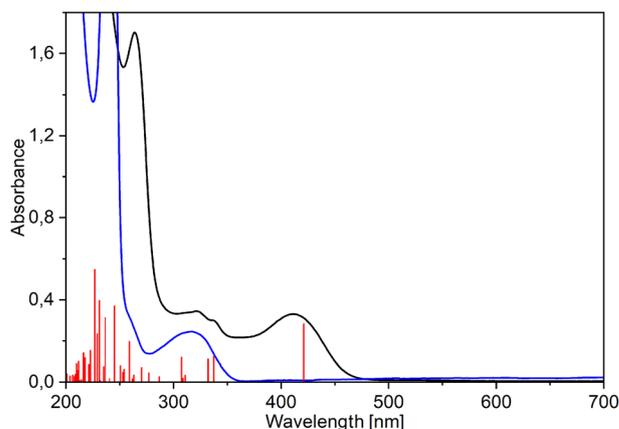
Fig. 4 Experimental (black) and TD-PBE0/def2-TZVP/IEFPCM (methanol) simulated (red vertical lines) UV-Vis spectra of  $[\text{Re}(\text{CO})_3(\text{Q})\text{Him}]$  (**1**) compared with the spectrum of 8-hydroxyquinoline (blue).
