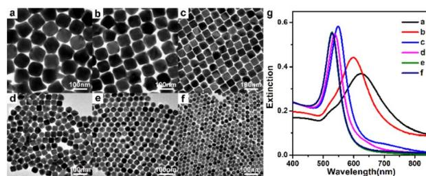
Fig. 1 TEM images (a to f) and the corresponding UV-vis absorption spectra (g) of the Au nanocubes produced at the seed volume of 3  $\mu$ L, 5  $\mu$ L, 10  $\mu$ L, 30  $\mu$ L, 50  $\mu$ L, and 80  $\mu$ L. The concentrations of CTAB, HAuCl<sub>4</sub>, and AA in the reaction mixture are 15 mM, 0.19 mM, and 8.8 mM, respectively.
