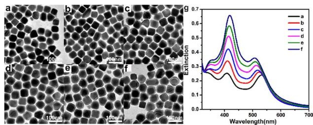
Fig. 2 TEM images (a to f) and UV-vis absorption spectra (g) of Au@Ag core-shell nanocubes with different Ag shell thicknesses obtained under different AgNO<sub>3</sub> concentrations, the AgNO<sub>3</sub> concentrations from (a) to (f) are 15 μM, 22 μM, 29 μM, 36 μM, 44 μM, and 51 μM, respectively.
