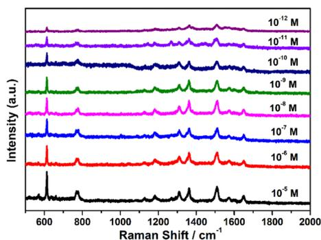
Fig. 4 Determination of SERS detection limit. Various SERS spectra of Au@Ag<sub>8.4</sub> nanocubes with respect to varied concentrations of R6G molecule (from  $1 \times 10^{-12}$  to  $1 \times 10^{-5}$  M).
