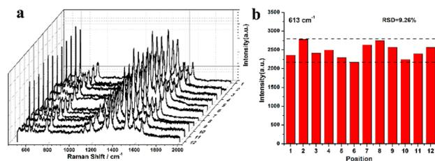
Fig. 5 Raman spectra of R6G at  $1 \times 10^{-6}$  M from 12 arbitrarily selected spots on the Au@Ag<sub>8.4</sub> nanocubes substrate (a). The histogram characterization of the intensities at the  $613 \text{ cm}^{-1}$  peak derived from Raman spectra (b).
