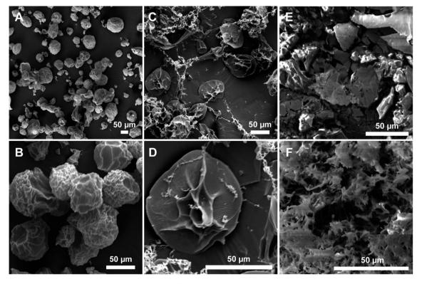
Fig. 3 SEM images of: (A and B)  $\kappa$ -c beads after spin-drying; (C and D)  $\kappa$ -c beads after vacuum drying; and (E and F) multicore capsules of  $\kappa$ -c beads in chitosan after vacuum drying
