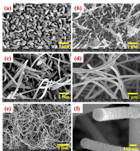
Fig. 3 FESEM images of (a) as-deposited Zn thin films and as-grown ZnO films after oxidation at (b) 500 °C for 5 h, (c) 600 °C for 5 h and (d) 700 °C for 30 minutes. (e) Large scale and (f) closer view of samples shown in (d).
