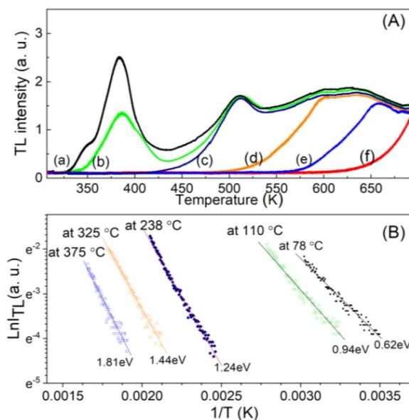
Fig. 4 (A) The obtained TL glow curves using the partial thermal-cleaning technique with  $T_{\text{stop}}$  (a)  $30\text{ }^{\circ}\text{C}$ , (b)  $60\text{ }^{\circ}\text{C}$ , (c)  $110\text{ }^{\circ}\text{C}$ , (d)  $230\text{ }^{\circ}\text{C}$ , (e)  $320\text{ }^{\circ}\text{C}$  and (f)  $380\text{ }^{\circ}\text{C}$ . (B) The graph of  $\ln I$  with  $1/T$  corresponds to 15% of the initial rise part of the TL curves of the low-temperature peaks (in (A)).
