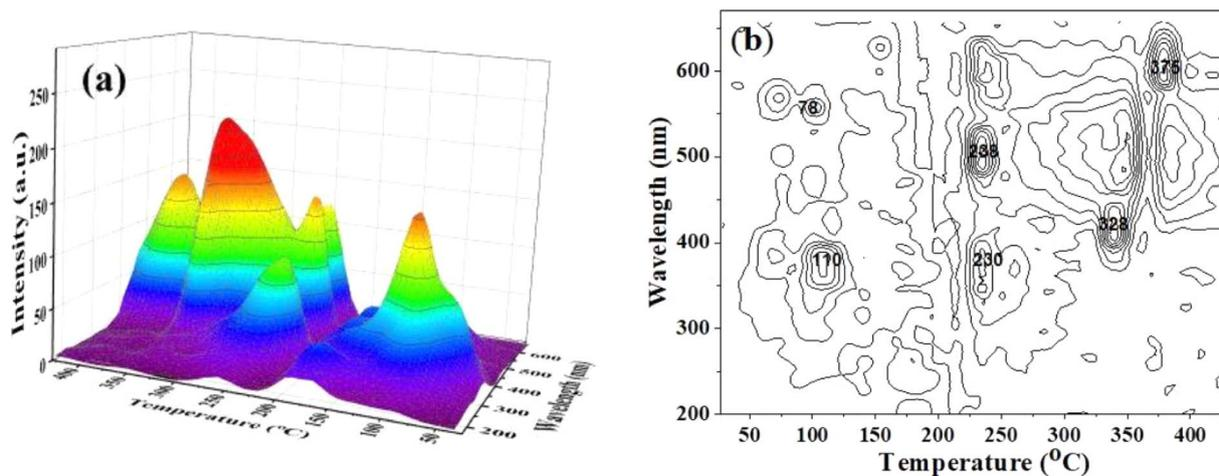
Fig. 3 3-D TL spectrum (a) and contour plot (2D-TL) of the emission spectrum (b) of the natural quartz (with the heating rate of  $\beta = 5\text{ }^{\circ}\text{C s}^{-1}$ ,  $\gamma$ -ray irradiation  $D\gamma = 6.4\text{ Gy}$ ).
