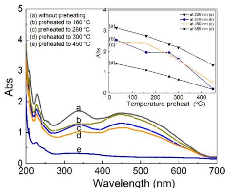
Fig. 12 Absorption spectra of natural quartz irradiated with a gamma dose of 19.2 Gy, measured under different preheated conditions (a) no preheated, (b) preheated to 160 °C, (c) preheated to 260 °C, (d) preheated to 300 °C, (e) preheated to 450 °C.
