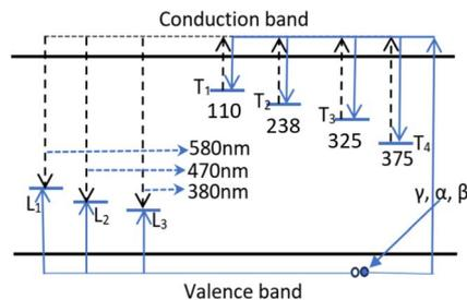
**Fig. 9** The energy band diagram for the kinetics of charge carriers in the TL process:  $T_{1,2,3,4}$  symbols are electron traps;  $L_{1,2,3}$  symbols are hole traps; solid arrows ( $\rightarrow$ ) indicate the movement of carriers during irradiation and dashed arrows ( $\dashrightarrow$ ) illustrate the carrier movement during heating.
