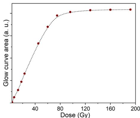
Fig. 14 The response of absorption *versus* irradiation dose (area under the curve).
