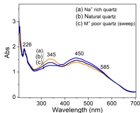
Fig. 13 Absorption spectra of natural quartz irradiated with gamma dose of 19.2 Gy (a) Na<sup>+</sup> rich quartz sample, (b) natural quartz sample and M<sup>+</sup> poor quartz sample.
