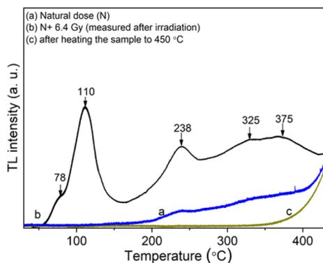
Fig. 2 The TL glow curve of the natural quartz in the region of the temperature from RT to 430 °C with the heating rate of  $\beta = 5\text{ °C s}^{-1}$ ,  $\gamma$ -ray irradiation ( $D\gamma = 6.4\text{ Gy}$ ).
