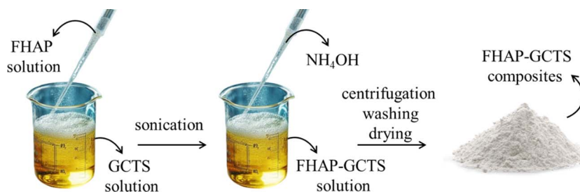
Scheme 2 Preparation of fish scale hydroxyapatite–gamma chitosan composites (FHAP–GCTS).
