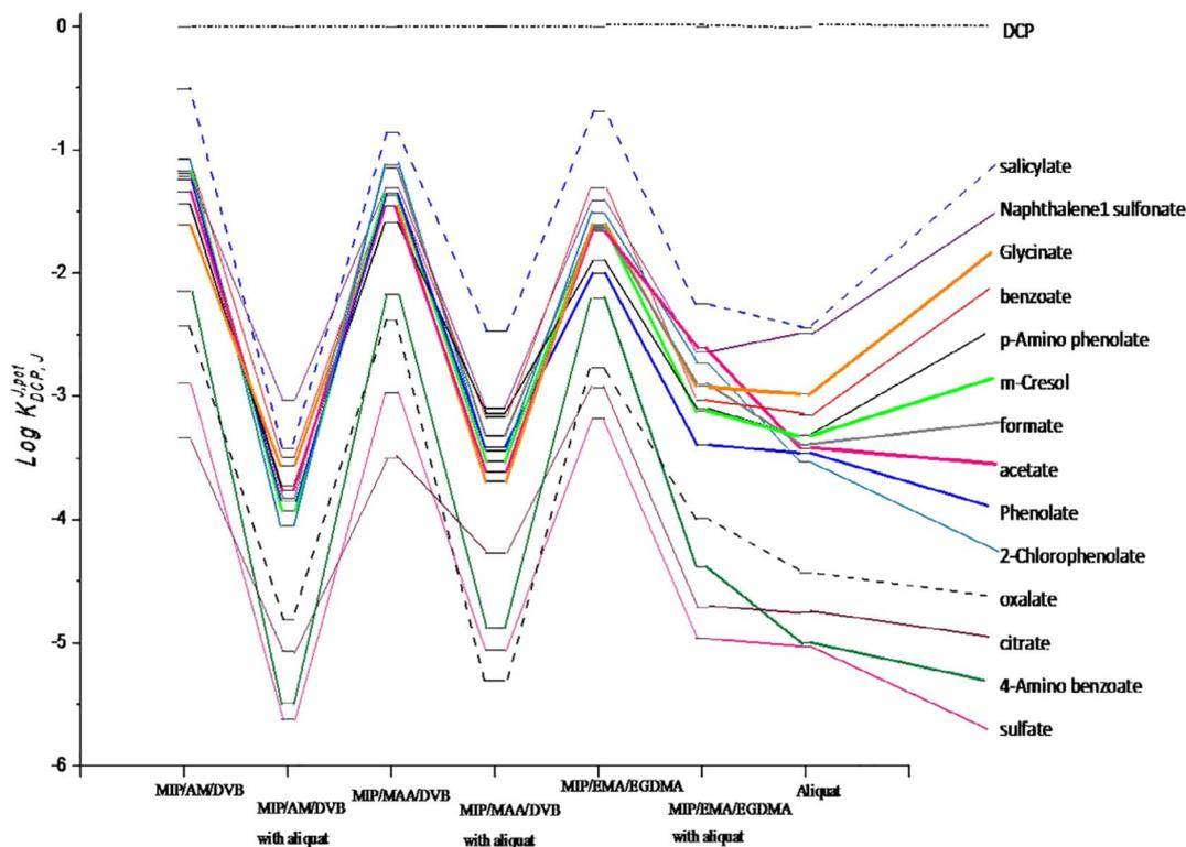
Fig. 14 Potentiometric selectivity coefficients  $\log K_{DCP,J}^{pot}$  of DCP membrane-based sensors.<sup>81</sup>
