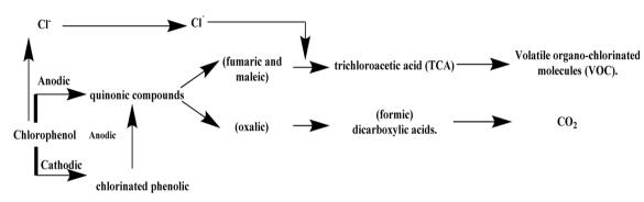
Fig. 21 A diagram illustrating the basic mechanistic model suggested to describe the primary procedures involved in the electrochemical treatment of CP wastes.
