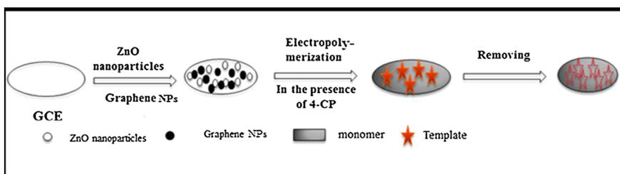
Fig. 6 Fabrication of the GCE/ZnO/GNPs/MIP.<sup>72</sup>
