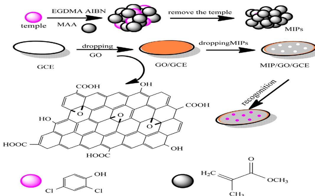
Fig. 11 Construction of the improved electrode and synthesis of the molecularly imprinted polymer.<sup>75</sup>
