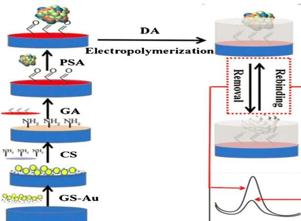
Fig. 3 Schematic of the fabrication and detection principle of the voltammetric MIP-based sensor towards PSA.<sup>56</sup>
