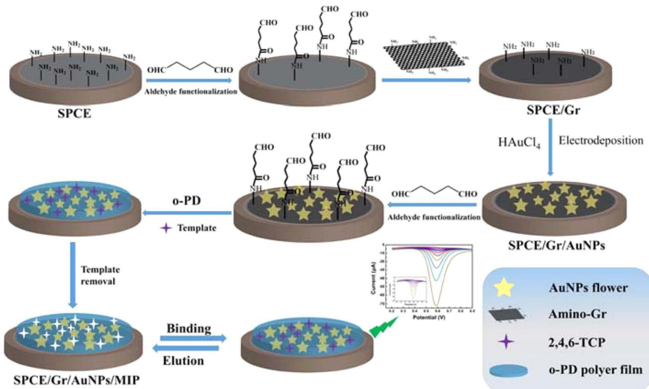
Fig. 15 An illustration of the steps involved in fabricating the SPCE/Gr/AuNP/MIP electrode.<sup>86</sup>
