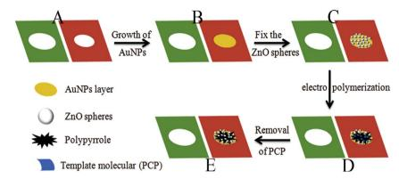
Fig. 20 Paper-based PEC sensor's manufacturing process.<sup>93</sup>
