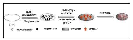
Fig. 6 Fabrication of the GCE/ZnO/GNPs/MIP.72
