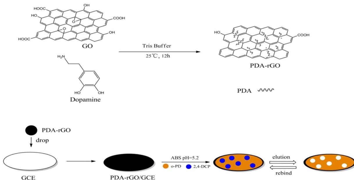
Fig. 9 Synthesis procedure for molecularly imprinted polymer and the modified electrode construction process.<sup>77</sup>
