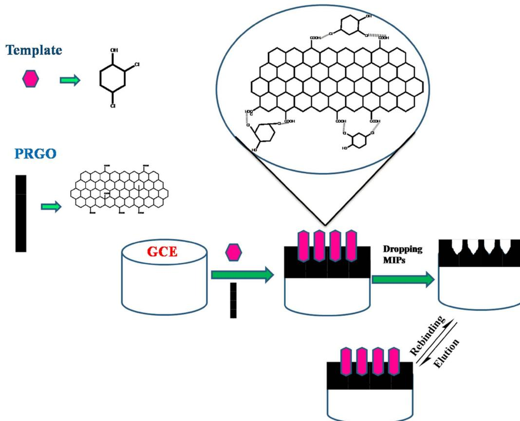
Fig. 13 Schematic representation for the fabrication of the MIP/PRGO microgel/GCE modified surface.<sup>80</sup>
