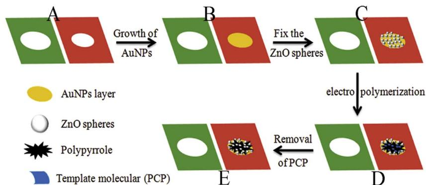
Fig. 20 Paper-based PEC sensor's manufacturing process.<sup>93</sup>
