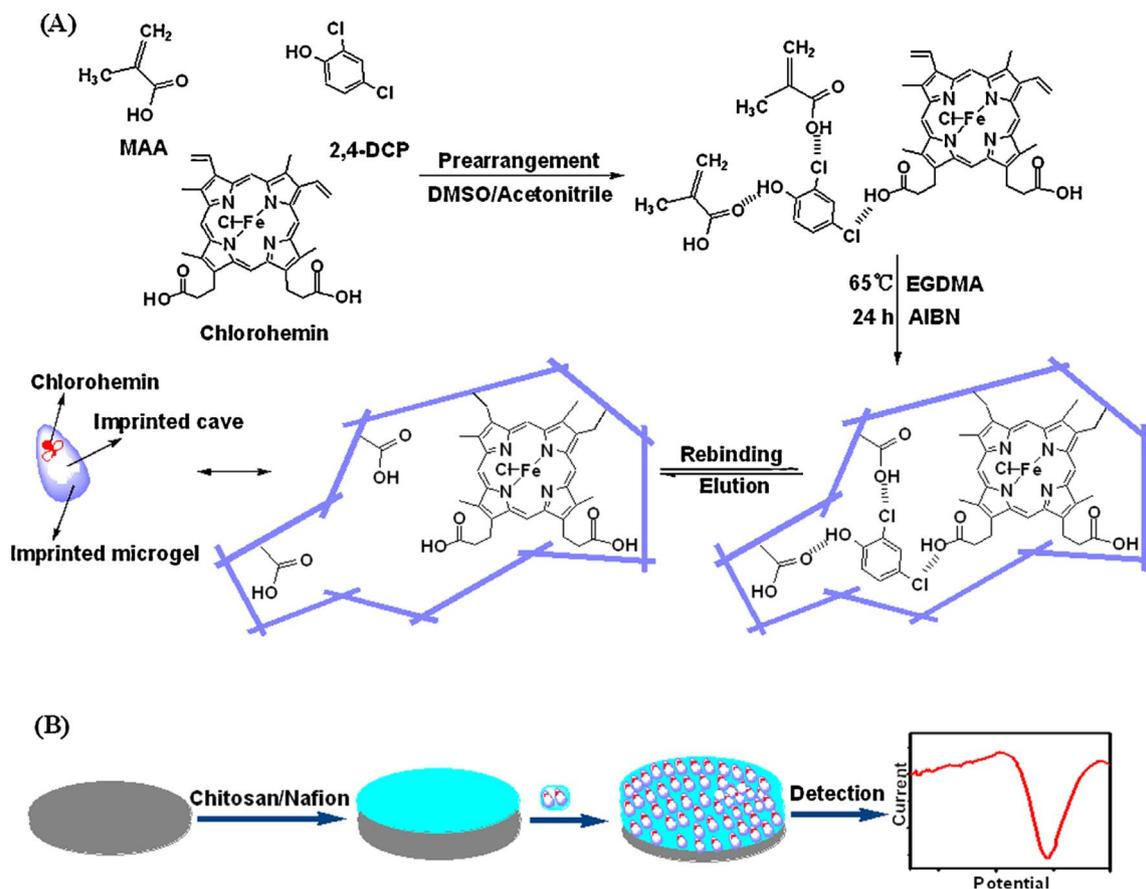
Fig. 12 Diagram showing the synthesis pathway of the 2,4-DCP imprinted microgel (A) and the fabrication of the imprinted sensor (B).<sup>79</sup>
