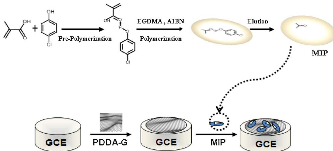
Fig. 7 Schematic illustration of the fabrication of MIP/PDDA-G/GCE.<sup>73</sup>
