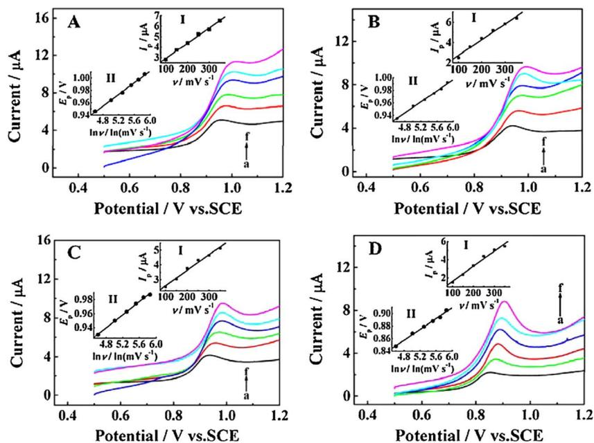
Fig. 17 Linear sweep voltammograms of 0.5 mM 2-CP (A), 4-CP (B), 2,4-DCP (C) and 2,4,6-TCP (D) in pH 2.56 BR buffer acquired at CS@Ag@GO/GCE with different scan rates ( $\nu$ ) of 100 (a), 150 (b), 200 (c), 250 (d), 300 (e) and 350 (f)  $\text{mV s}^{-1}$ . Insets: (I) peak current ( $I_p$ ) versus  $\nu$ . (II) Peak potential ( $E_p$ ) versus  $\ln \nu$ .<sup>88</sup>
