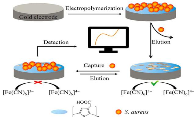
Fig. 2 Schematic of the sensing approach for *S. aureus* sensing based on an electropolymerized MIP.<sup>55</sup>
