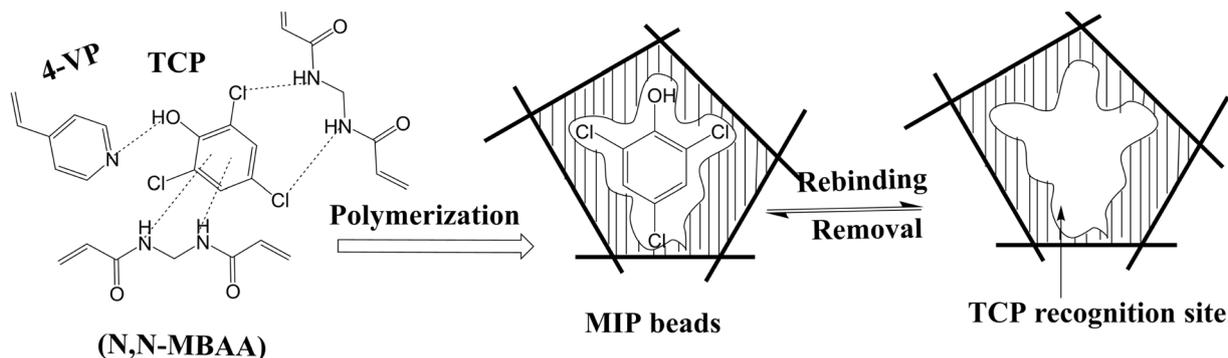
Fig. 18 Schematic diagram of the imprinting process of TCP/MIP.<sup>85</sup>
