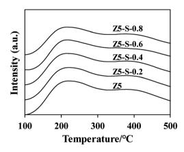
Fig. 3 NH<sub>3</sub>-TPD curves of CLD samples.
