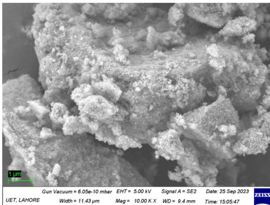
Fig. 4 SEM analysis of the TiO<sub>2</sub> nanoparticles. The SEM image clearly exhibits the morphology of the TiO<sub>2</sub> nanoparticles which is a spherical agglomeration that is homogenously distributed through the entire surface.
