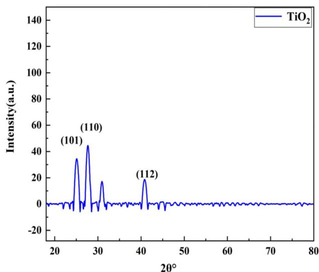
Fig. 3 XRD analysis of the TiO<sub>2</sub> nanoparticles.
