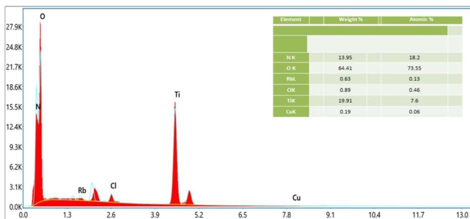
Fig. 5 EDX spectrum of the TiO<sub>2</sub> nanoparticles. Peaks representing pure titanium and oxygen are present in the specimen.
