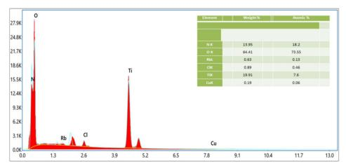
Fig. 5 EDX spectrum of the TiO<sub>2</sub> nanoparticles. Peaks representing pure titanium and oxygen are present in the specimen.
