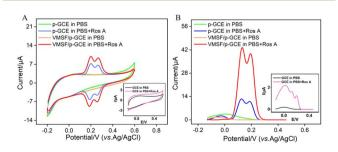
Fig. 5 CV curves (A) and DPV curves (B) obtained on different electrodes in 0.1 M PBS (pH = 7) without or with Ros A (20  $\mu$ M) at a scan rate of 50 mV s<sup>-1</sup>. Insets show the corresponding CV or DPV curves obtained on GCE in the presence or absence of Ros A.
