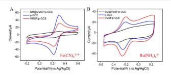
Fig. 4 CV curves obtained on different electrodes in Fe(CN) $_6^{3-/4-}$  (A) or Ru(NH $_3$ ) $_6^{3+}$  (B) solution.
