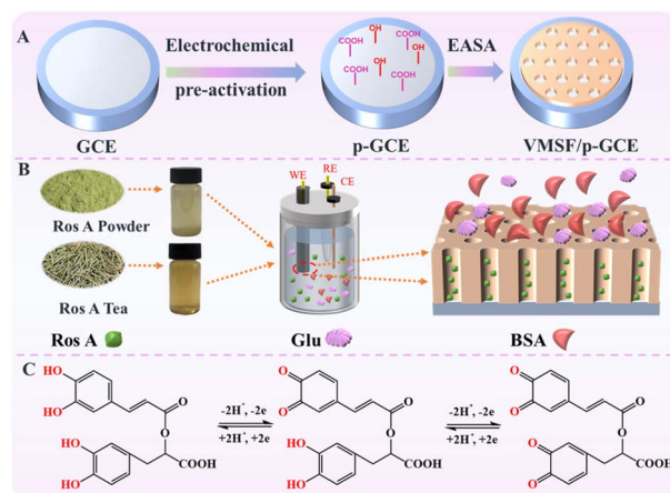
Fig. 1 Schematic illustration for the fabrication of VMSF/p-GCE sensor (A), the anti-fouling/anti-interference properties of nanochannel in real sample (B) and the electrochemical process Ros A on electrode (C).
