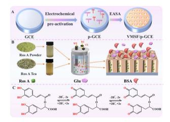
Fig. 1 Schematic illustration for the fabrication of VMSF/p-GCE sensor (A), the anti-fouling/anti-interference properties of nanochannel in real sample (B) and the electrochemical process Ros A on electrode (C).
