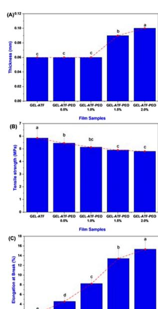
Fig. 4 Differences in thickness (A), tensile strength (B), and elongation at break (C) of gelatin-arrowroot tuber flour (GEL-ATF)-based edible films with and without added pomelo pericarp essential oil (PEO) at varying concentrations. Different letters in the graph indicate significant differences between the means (P < 0.05).
