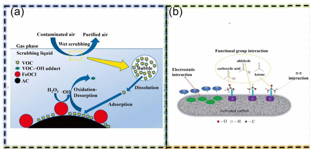
Fig. 2 (a) Schematic illustration of DCE removal by wet scrubbing using  $FeOCl/AC$ .<sup>36</sup> (b) The possible mechanism of  $Mn^{2+}$  adsorption over  $AC$ <sup>36</sup> (this figure has been reproduced with permission from Najm *et al.*<sup>35</sup> from Elsevier, copyright 2020).
