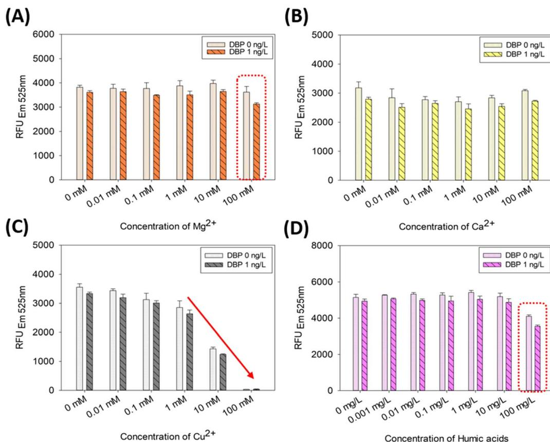
Fig. 5 DBP quantification using the SG-aptasensor in the presence of environmental inhibitors: (A) Mg<sup>2+</sup> ion, (B) Ca<sup>2+</sup> ion, (C) Cu<sup>2+</sup> ion, and (D) humic acids.
