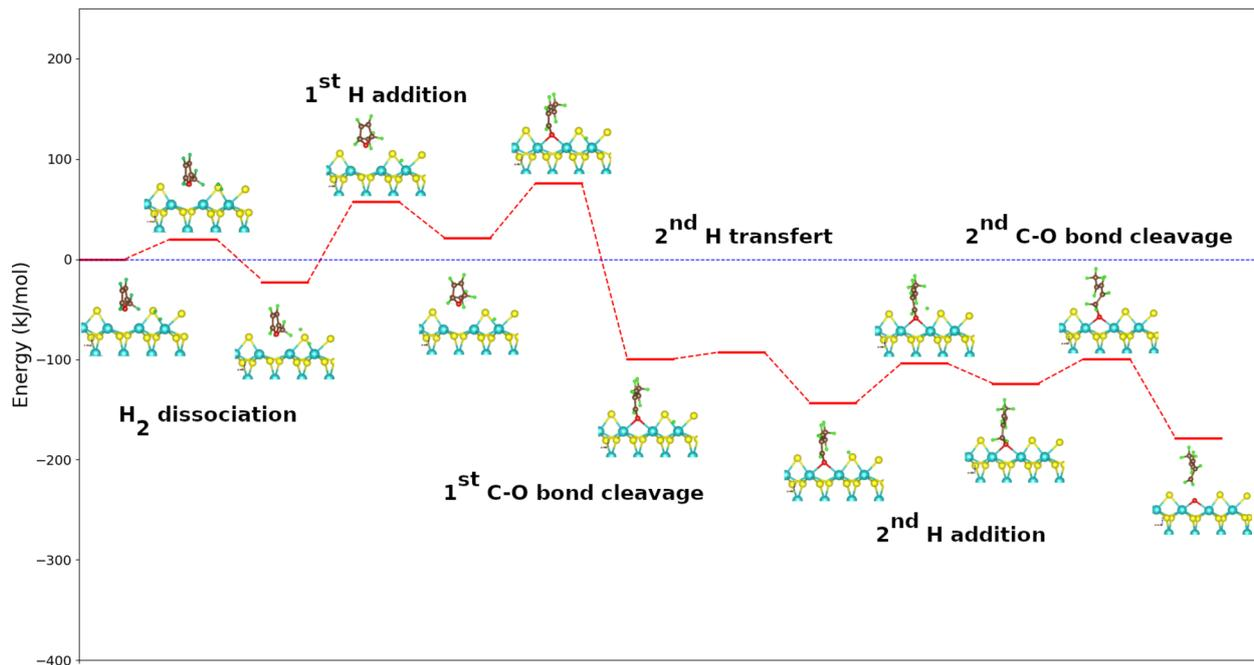
Fig. 4 Energy diagram of DDO (5H) route of the 2-methylfuran molecule on the metal edge of MoS<sub>2</sub> surface using the PBE + D2 approximation. For clearer images, please refer to Fig. S4 in the ESI.†
