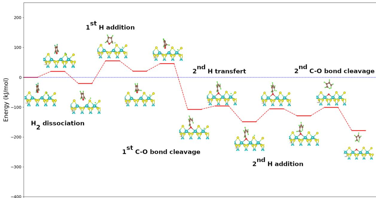
Fig. 2 Energy diagram of the DDO route of furan on the metal edge of MoS<sub>2</sub> surface using the PBE + D2 approximation. For clearer images, please refer to Fig. S6 in the ESI.†
