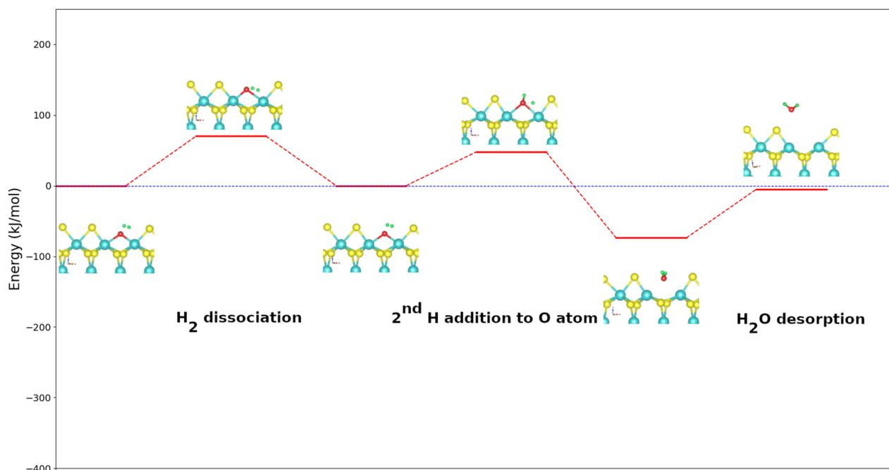
**Fig. 3** Energy diagram for vacancy regeneration on the metal edge of MoS<sub>2</sub> surface after oxygen atom removal from the studied molecules. For clearer images, please refer to Fig. S3 in the ESI.†
